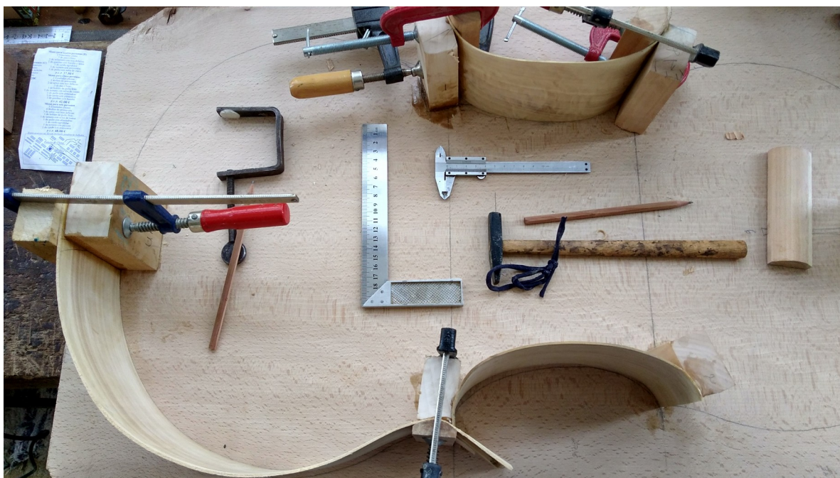
The “freestyle” construction of our bass violin directly on the back, without using an internal mold
