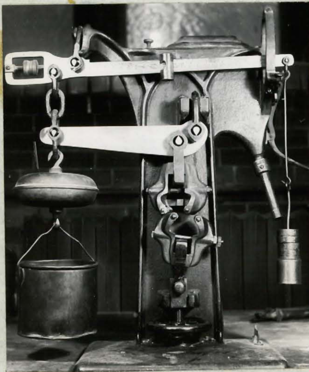
Photograph No. 3 - Specimen broken, lead shot being weighed to deter- mine rupture stress value.
