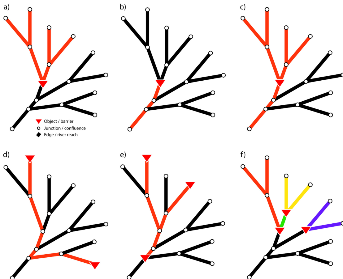
Figure 1.4: Schematic river network illustrating routing functions currently implemented in HydroROUT: a) upstream routing, selecting all reaches upstream of an object/barrier (red triangle); b) downstream routing; c) combined upstream/downstream routing; d) find shortest connected path between two objects; e) shortest path between multiple objects (minimum spanning tree); and f) routing with multiple barriers ('find all connected').
