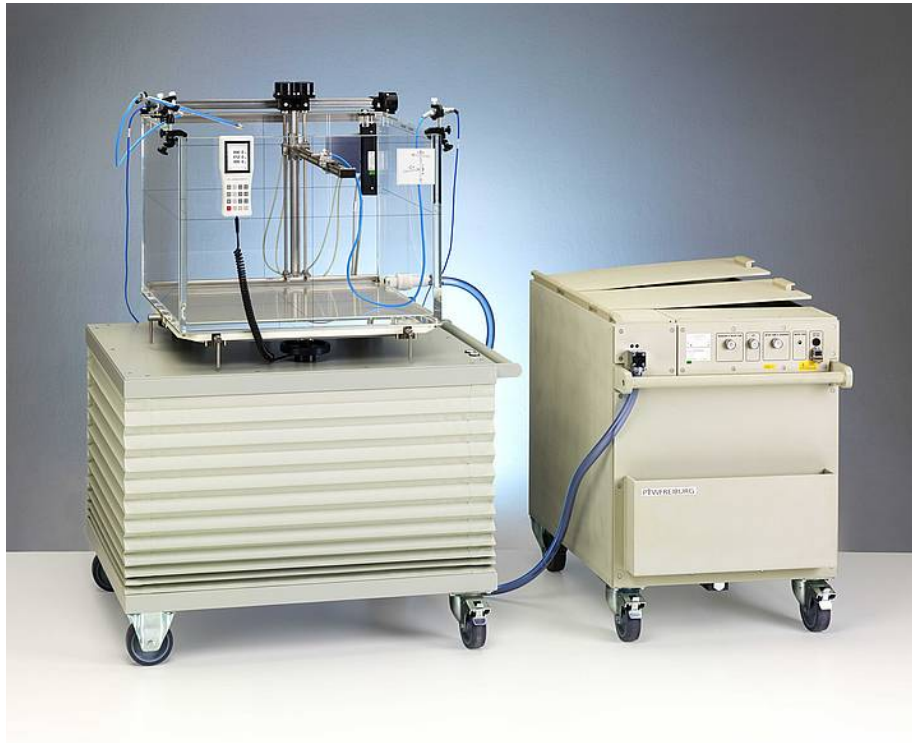
Figure 1–2: Picture of a PTW Freiburg MP3 scanning water tank system [9]. Shown on the picture are the water tank itself on a vertically-adjustable platform and the water reservoir and pump systems on the right.
