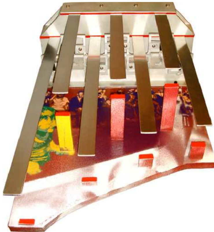
Fig. 4.1 Archival photo (IDMIL Laboratory Library) of The Rulers: a Digital Musical Instrument, a set of seven cantilever beams designed to evoke deflection gestures. Photo and design by David Birnbaum.
