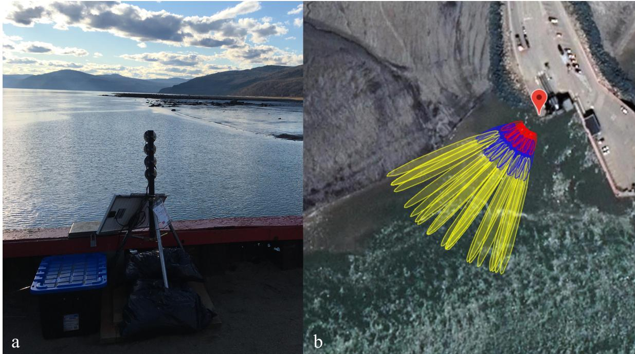
**Figure 4.3:** a) A Picture of the site at Saint-Joseph-de-la-Rive and b) a top-down view of the reflection zones from <https://gnss-reflections.org/rzones> (Roesler and Larson, 2018). In the left picture, the stilling well that contains the pressure gauge can be seen to the left of the tripod, with a padlock attached to it. The different coloured ellipses refer to reflection zones from satellites at an elevation of 5, 10 and 15 degrees (yellow, blue and red, respectively).
