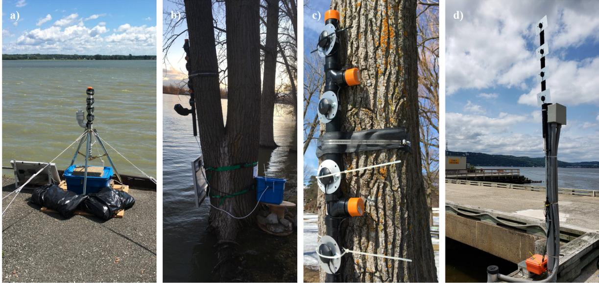
**Figure 3.3:** Pictures of antenna arrays a) at Trois-Rivières, b) and c) show different angles at Sainte-Anne-de-Bellevue and d) at Piermont. The antenna array showed in b) and c) was also temporarily installed at Trois-Rivières. The antennas are closer together in a) in comparison to the other two setups.
