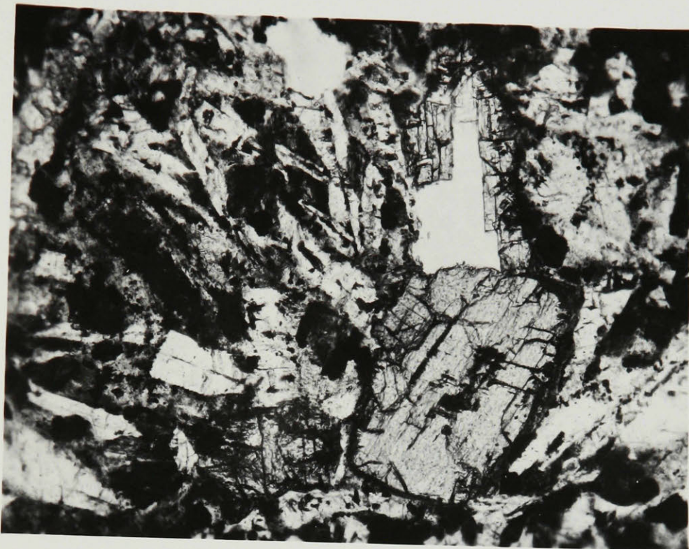
Fig. 8. Specimen No. 49-21. Diabase eight feet from south contact; shows unique occurrence of fresh augite. Magnification 80 X. Uncrossed nicols.
