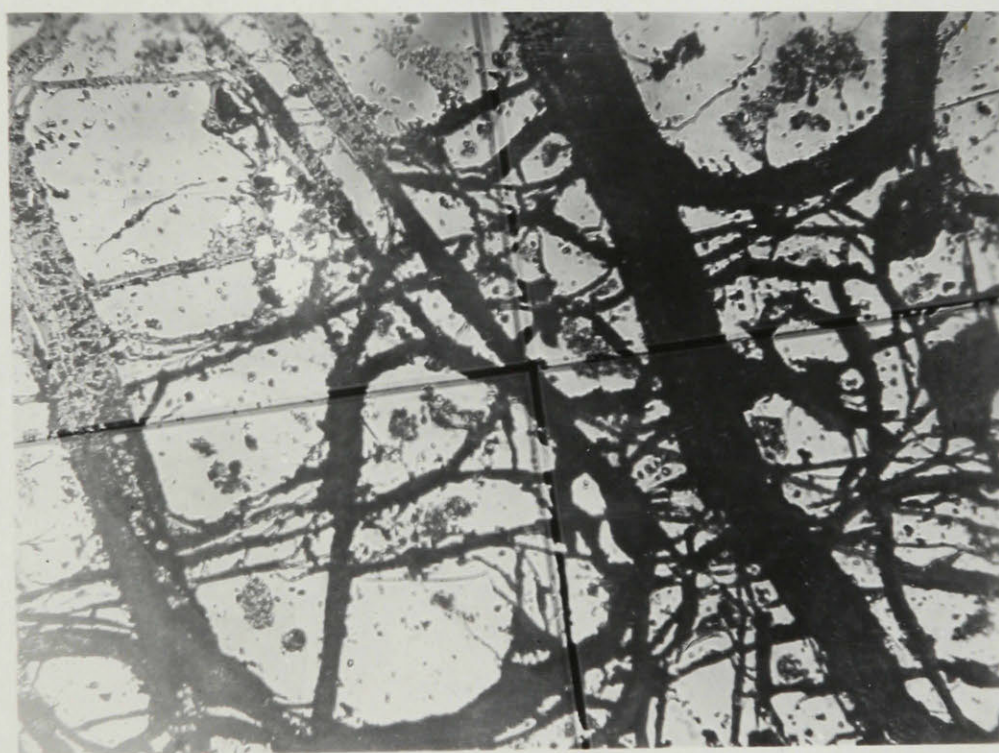
Fig. 19. Colloform pitchblende crossed by ramifying veinlets of calcite. Pyrite (white) in upper left. Magnification 20 X. Plain light.
