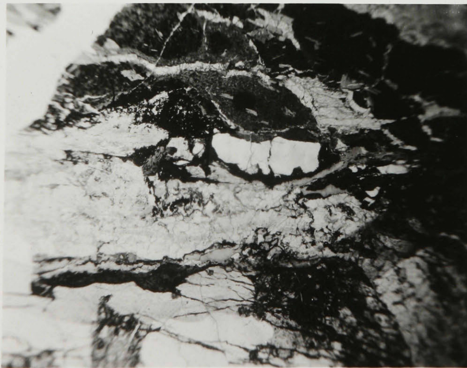
Fig. 13. Specimen No. 49-16. Breccia from south contact showing fractured quartz fragments, and partial replacement of diabase by hematite. Magnification 18 X. Uncrossed nicols.
