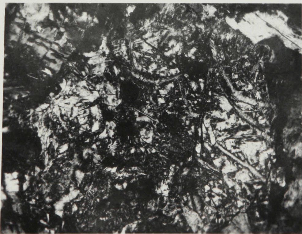
Fig. 9. Specimen No. 49-31. Diabase from center of dyke. Photomicrograph shows aggregate of serpentine representing original olivine crystal. Magnification 80 X. Crossed nicols.
