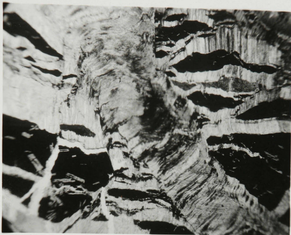
Fig. 12. Specimen No. 49-15. Breccia from south contact. Fragments are diabase replaced by opaque hematite with laths of chlorite pseudomorphous after plagioclase phenocrysts. Matrix is calcite and chlorite stained with hematite. Magnification 27 X. Uncrossed nicols
