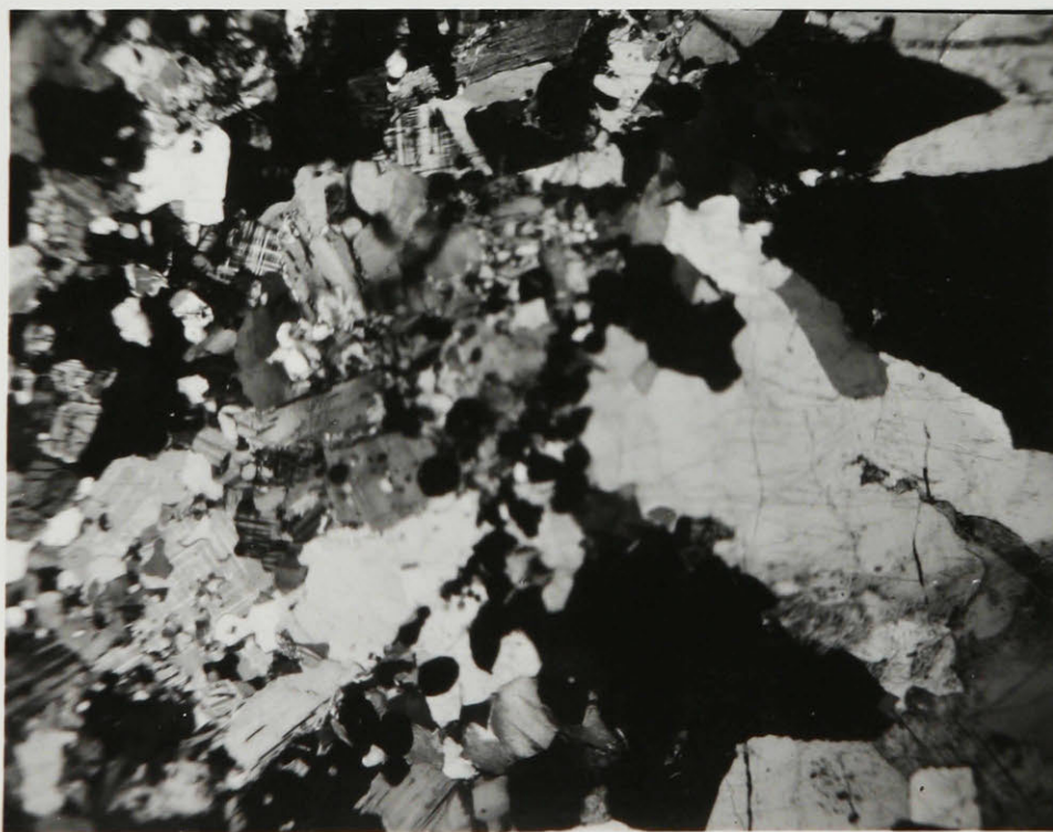
Fig. 18. Specimen No. 49-37. Granite from south contact. Zone of small garnet crystals divides area in two parts: left is fine-grained granite with much microcline; right is coarser, shows orthoclase replacing oligoclase. Magnification 35 X. Crossed nicols.
