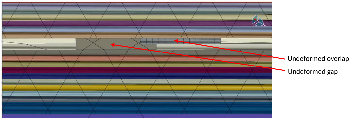
Figure 3.17: Cross section of the laminate before simulation
