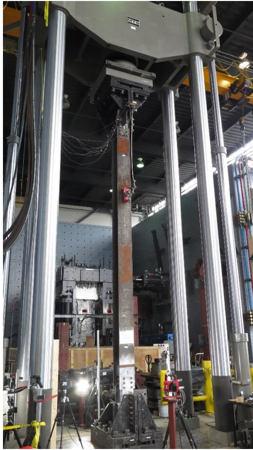
Figure 4.2: Test set-up of the full-scale I-shape brace and connection assembly [18,19]
