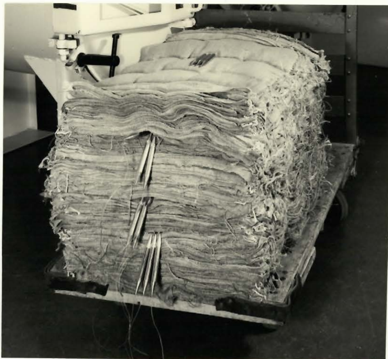
Figure 5. Bale of jute bags used in fumigation experiments, showing metal capsules containing insects ready for drawing into position within the bales.
