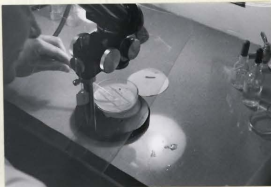
Suction removal of used antiseptic and debris from well slide.
