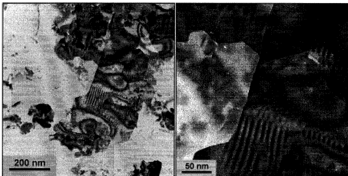
Figure 2: \text{AgNO}_3 SMA 50,000 Da reduced slowly with a dilute solution of \text{NaBH}_4 with a pH of 7. Lines are 3 nm in diameter. The darker areas are most likely reduced silver onto the inner or outer nanotube walls. The line diameter and spacing agree with the theoretical values predicted in Chapter II.
