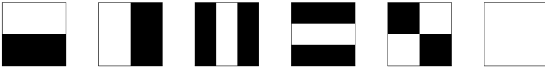
Figure 3.3 The match filters used in Chromaprint.
