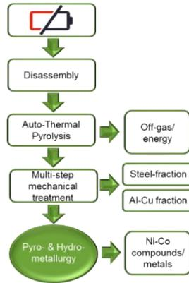
Supplementary Figure 6 Accurec Recycling GmbH LIB recycling process [1].
