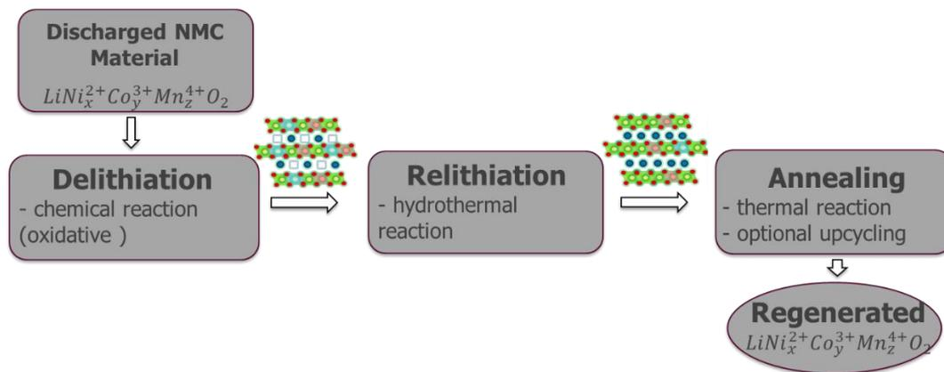
Figure 2-13 Typical Direct Recycling Process of LIBs Containing NMC Cathode
