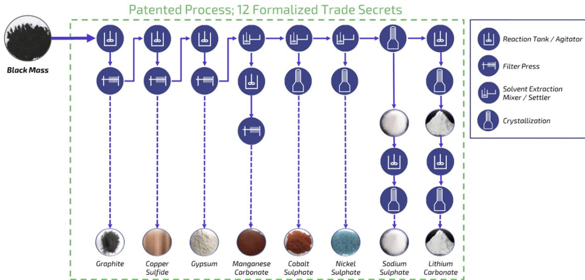
Figure 2-18 Li-Cycle Hydromet Process for Recycling lithium-ion batteries [68].
