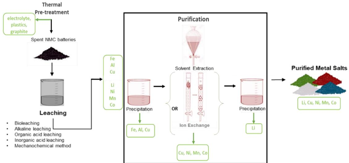
Figure 2-4 Recycling using hydrometallurgical processing, adapted with permission from [34].
