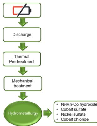
Supplementary Figure 4 Brupr LIB recycling process (adapted from [1]).
