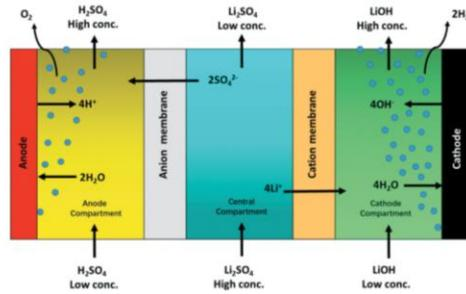
Figure 2-19 American Manganese RecycLiCo™ process, a three-compartment membrane electro dialysis cell for generating LiOH and H<sub>2</sub>SO<sub>4</sub> [70].
