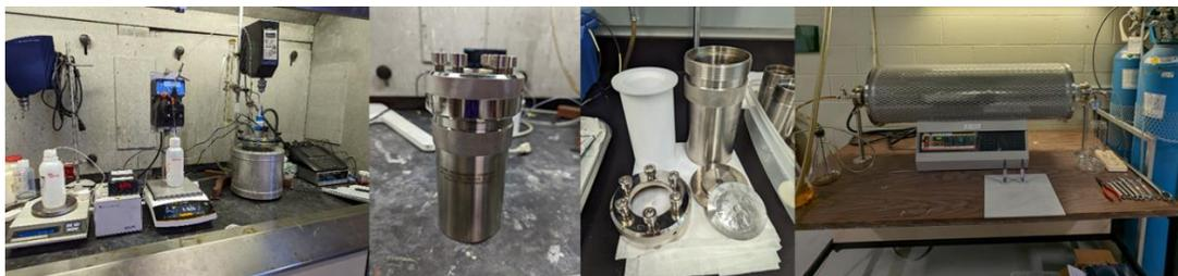
Figure 5-1 Delithiation set up (left) Hydrothermal reactor and Teflon liner insert (middle) and short annealing tube furnace (right).
