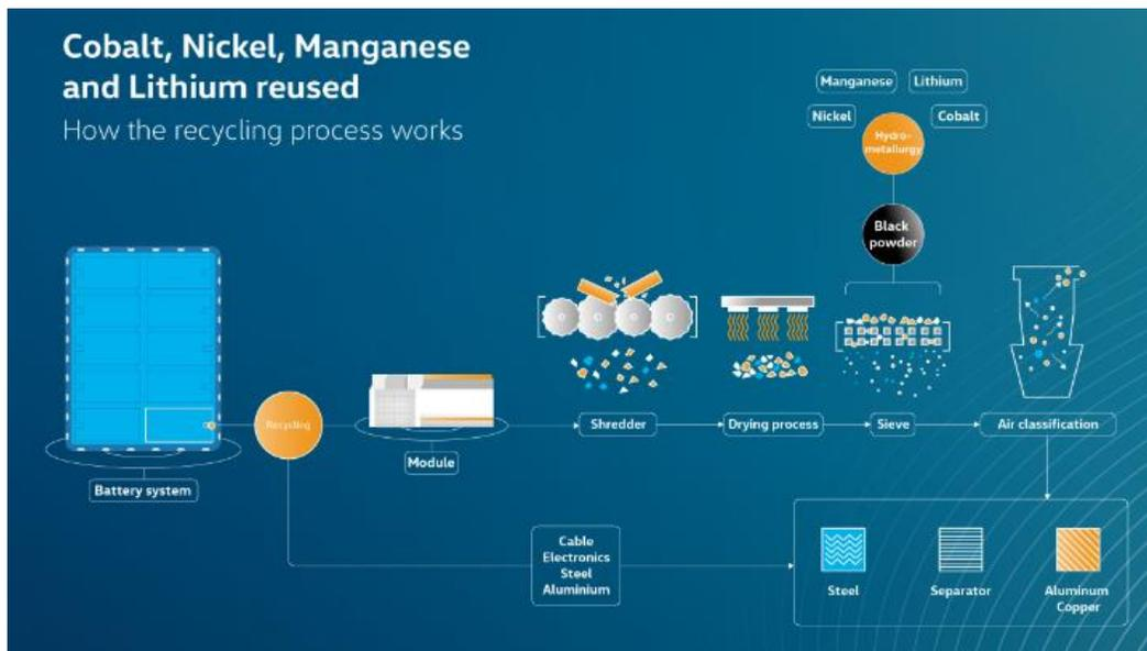
Supplementary Figure 10 Volkswagen adopted the LithoRec process for recycling LIBs [5].
