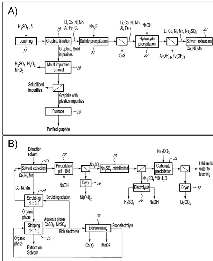
Figure 2-17 Lithion Recycling Patented Hydromet process (A) leaching circuit and (B) Metal separation for recovery of all value metals and graphite from spent NMC [66].
