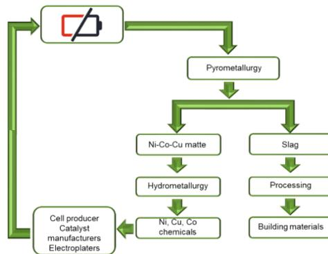
Supplementary Figure 7 Nickelhütte LIB recycling process [4].
