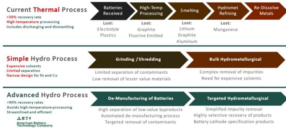
Figure 2-16 American Battery Technology streamlined recycling process [65].
