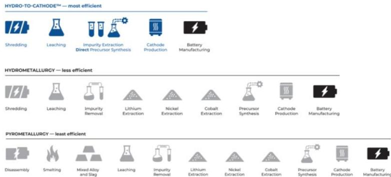
Figure 2-20 Ascend Elements (Battery Resourcers) LIB recycling process [72].
