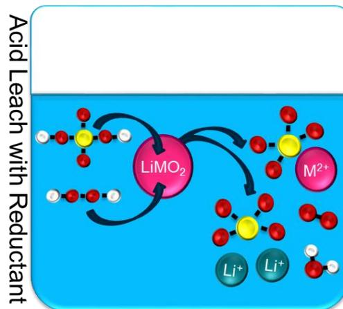
Figure 2-6 Typical Acid Leach with Reductant for NMC Recycling, where yellow = sulfur, red = oxygen, white = hydrogen, M = metal (Ni-Mn-Co), M<sup>2+</sup>= metal ions (divalent).
