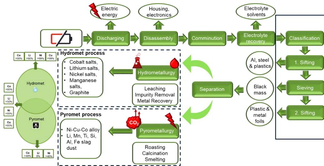
Figure 2-5 Lithium-ion battery recycling flowsheet overview comparing hydromet and pyromet processes
