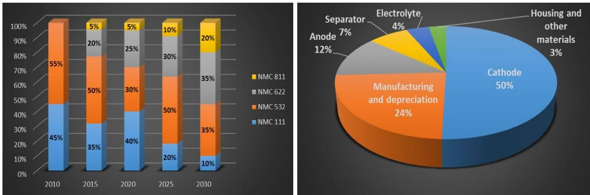
Figure 2-3 a) NMC cathode chemistry evolution [23], b) The cost of a lithium-ion battery [14]
