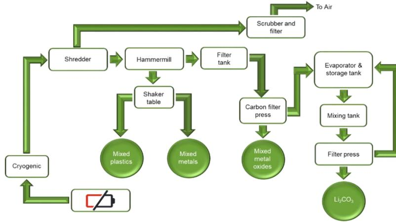
Supplementary Figure 1 Toxco recycling process (adapted from [2])
