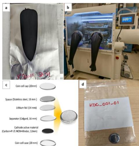
Figure 5-3 Coin cell battery assembly a) casting cathode onto aluminum foil b) assembly inside glove box c) coin cell fabrication schematic d) coin cell containing upcycled NMC 622 cathode material.
