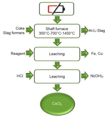
Supplementary Figure 3 Umicore LIB recycling process (adapted from [3])
