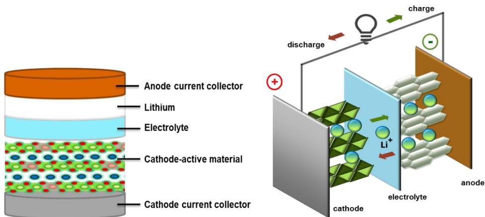
Figure 4-2. Lithium-ion battery schematic diagram (left), schematic of lithium-ion battery cell charging/discharging mechanism (right).
