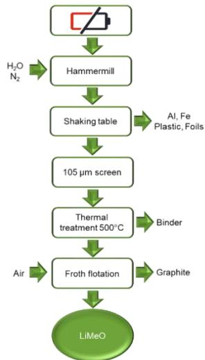
Supplementary Figure 2 Retrieval LIB recycling process for cathode-grade material regeneration (adapted from [3])
