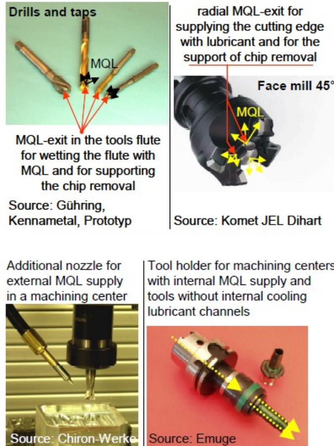
Figure 1.2 Different MQCL liquid delivery systems [3]
