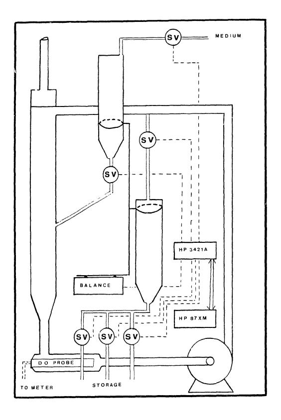
cycle time could be selected and any dosing or harvesting volume accurately obtained, independent of foaming. In addition, three sample valves could now be connected, extending the period of automatic operation before sample containers were replaced.
