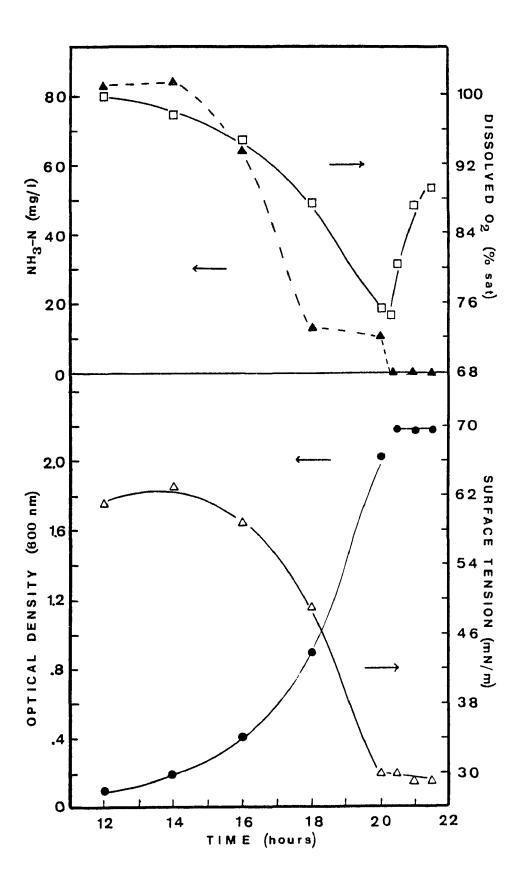
after about 18 hours. Figure 10 also illustrates the close correspondence between the maximum biomass concentration and minima in the surface tension, nitrogen and dissolved oxygen concentrations.
