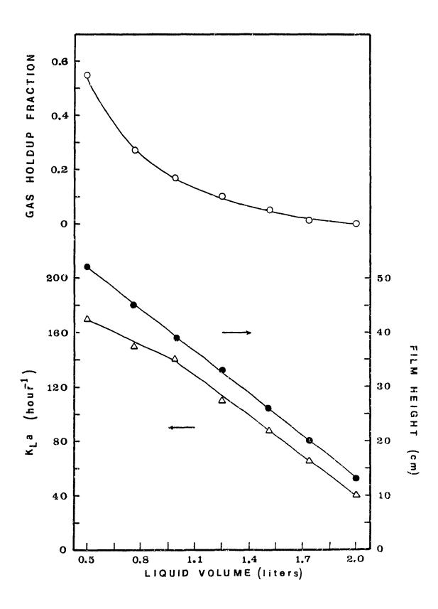
about 24 cm<sup>2</sup> or a maximum of 1300 cm<sup>2</sup> with a 500 mL working volume. The interfacial area provided by the entrained bubbles is not known since this requires measurement of the bubble size distribution.
