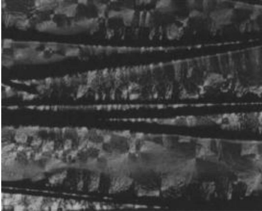
**FIGURE 2.2-2: SPHERULITIC AND EPITAXIAL CRYSTAL GEOMETRY FORMATIONS IN THE THERMOPLASTIC MATRIX OF A FIBER COMPOSITE [7]**
