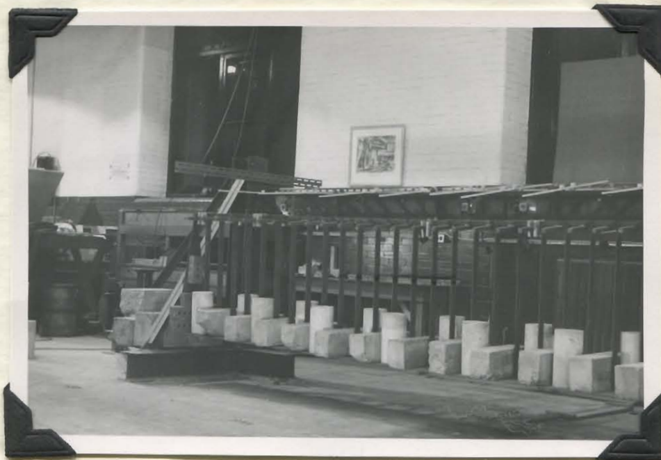
PHOTO IV. Left side view showing stand base and angle of twist when beam is loaded.
