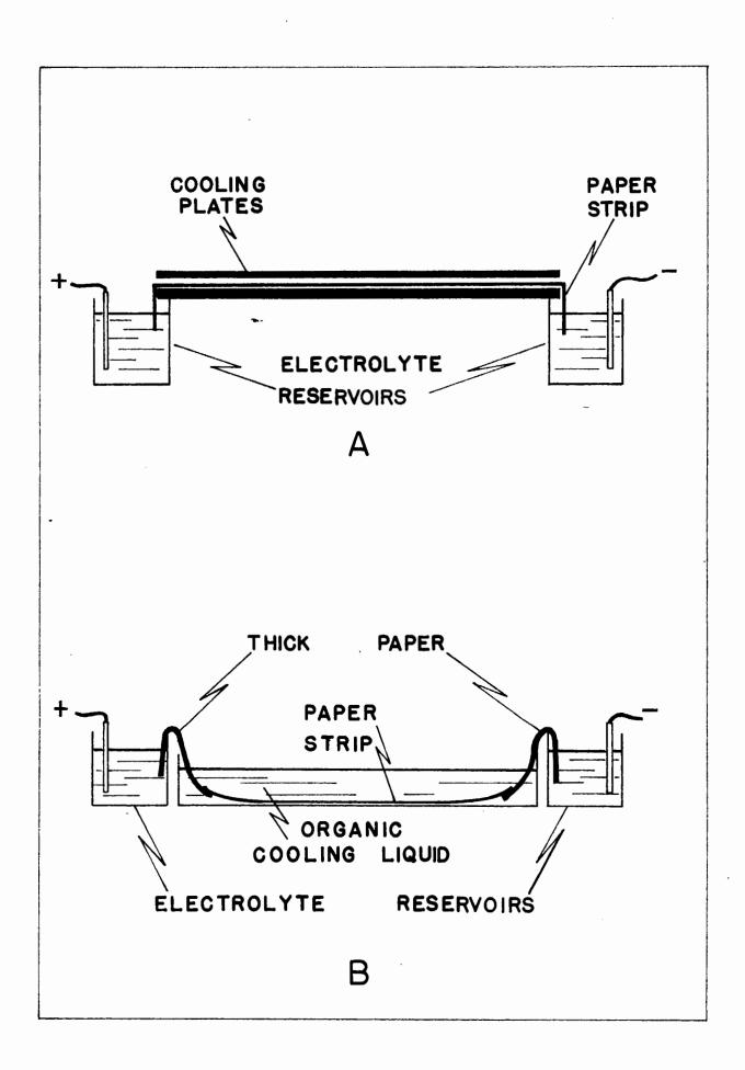
It has become customary to divide electromigration procedures arbitrarily into low and high voltage techniques. The latter generally refers to operation with a voltage gradient greater than about 20 volts per centimetre. There is of course no fundamental distinction, but the high voltage technique requires more careful attention to cooling. As a rule, all high voltage work must be done by a closed strip technique, although not all closed strip operation is a high voltage method.
