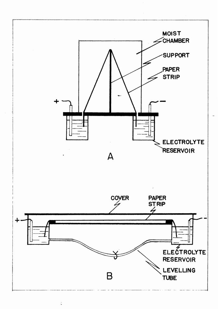
The strip is hung over the horizontal part of an inverted L-shaped glass rod, and the ends are allowed to dip into two vessels of background electrolyte solution which also contain the electrodes. These vessels are covered by a plastic plate containing slots for the ends of the strip, and a third vessel is inverted over the paper to form the moist chamber. Another popular arrangement (8,31), shown in primitive form in fig. 1B, has the strip pulled taut horizontally on a plastic frame.
