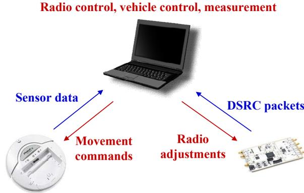
**Figure 3.13** The components of a DSRC-enabled vehicle and their connections.
