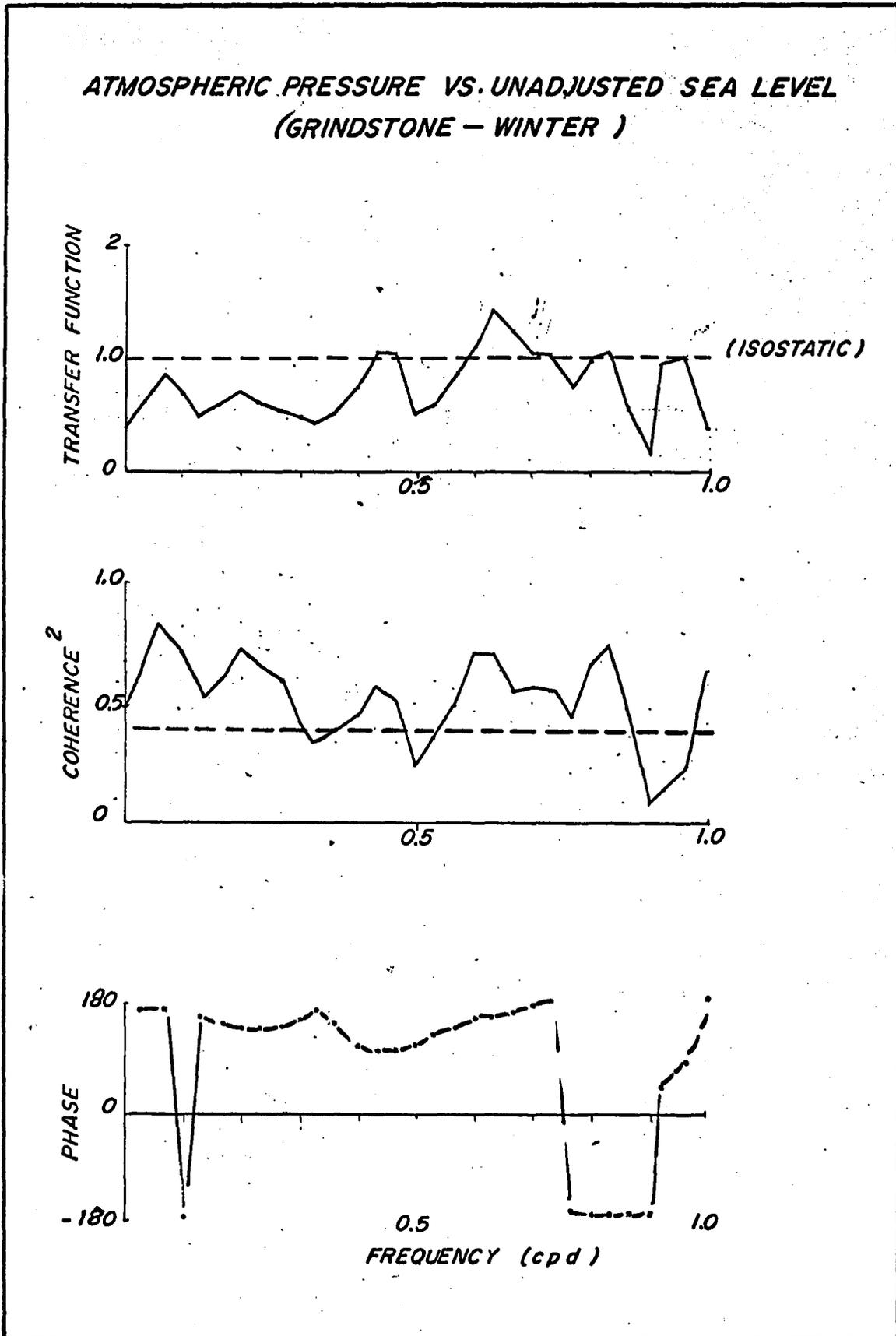
Fig. 20 Cross-spectrum between Sea Level and Atmospheric pressure
