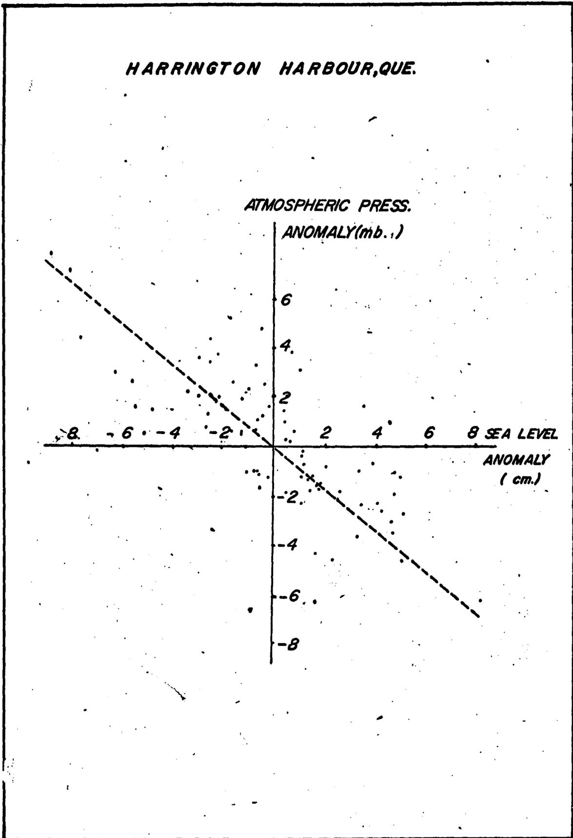
FIG. 6 Relation between Sea Level and Atmospheric Pressure at Harrington, Quebec
