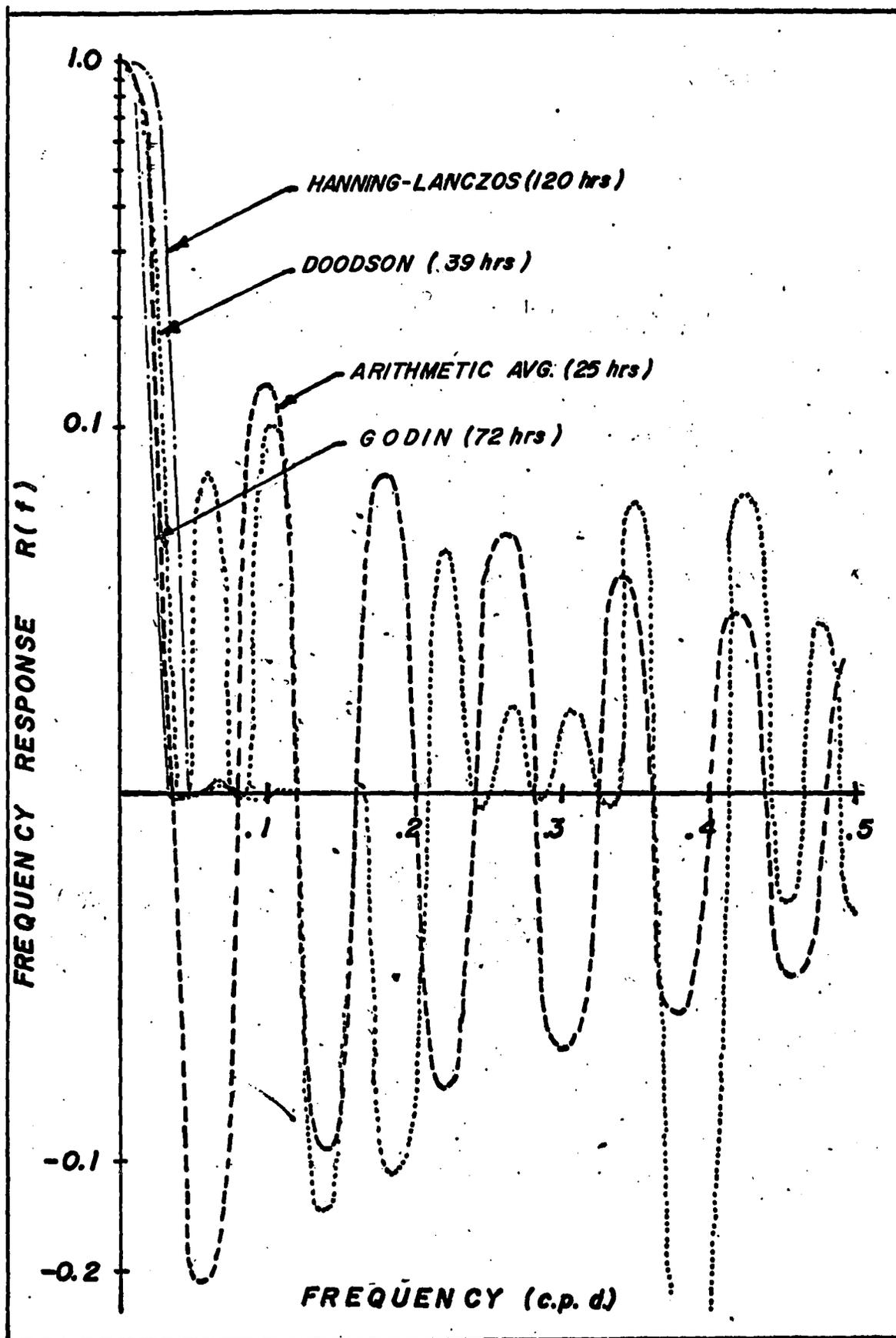
FIG. 12 Frequency Response characteristics of Tide filters
