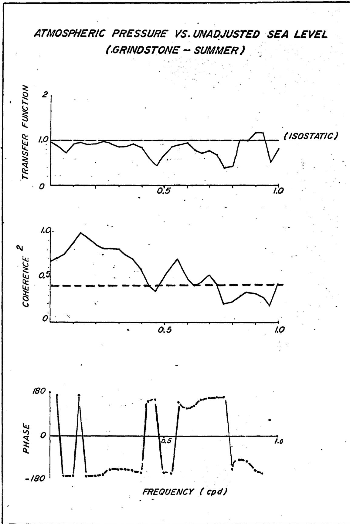
Fig. 19 Cross-spectrum between Sea Level and Atmospheric Pressure
