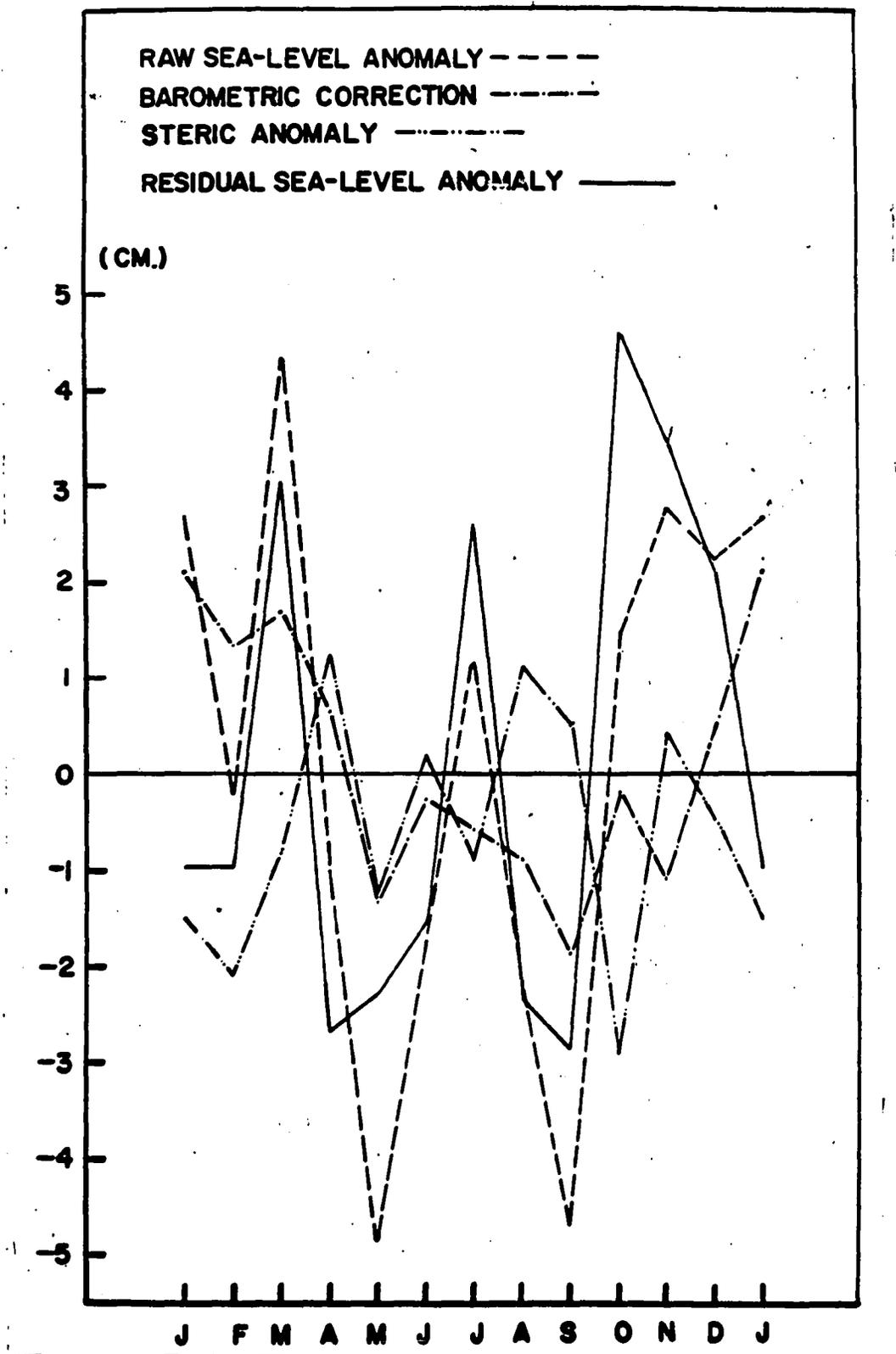
Figure 9 - Time series of raw sea level, isostatic corrections, and residual sea level anomaly ( Port aux Basques )
