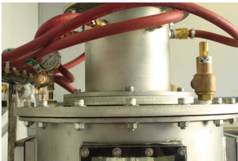
Figure 3.12: The pressure gauge and the release valve located on the top cover of the tank
