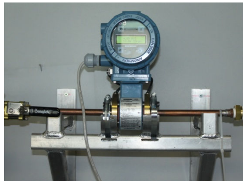
Figure 3.13: The magnetic flow-meter and its local operator interface
