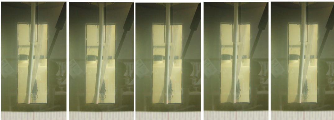
Figure 3.24: The motion of Pipe 1 in Configuration 3ii at U = 6.01 m/s
