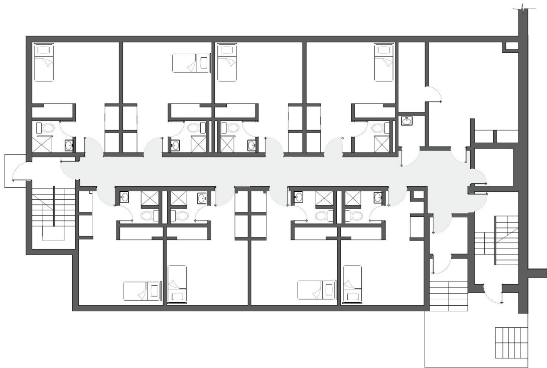
Figure 2.8: Typical floor plan of a rooming house. Logan House offers 13 dwellings destined for families and 26 SRO units for singles. SCALE 1:200. Adapted from House Design Guide for Low-Income Singles (p.290), by P. Teasdale, 1993, Ottawa: CMHC.
