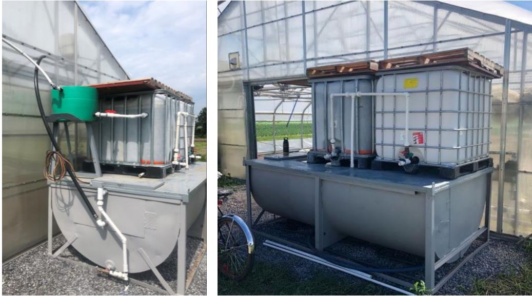
Figure 3: Final SSF system
