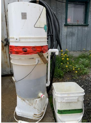
Figure 16. Small-Scale SSF Setup for Sand Testing
