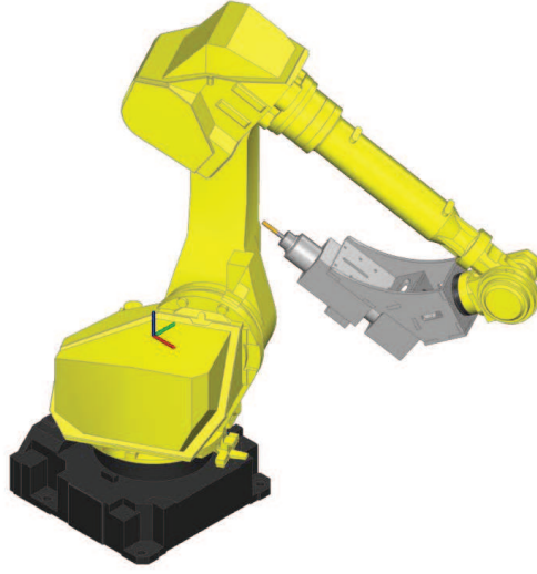
Figure 4-3: Optimum posture of the FANUC 710ic-50 with milling tool
