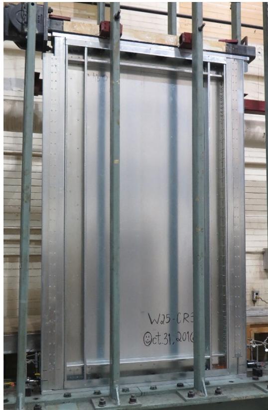
Figure B-15 Centre-sheathed configuration: W25-R3
