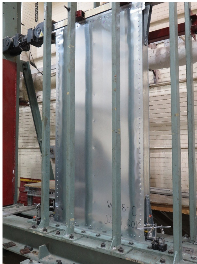
Figure 2.15 Double-sheathed configuration: specimen ready to be tested
