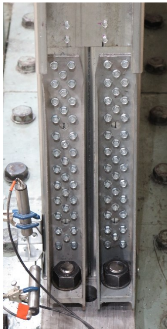
Figure B-12 Centre-sheathed configuration: bottom holdowns (a. & b.) and c. corner of W18-R
