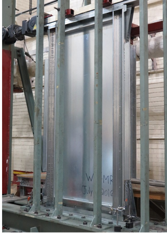
Figure B-11 Centre-sheathed configuration: W18-R
