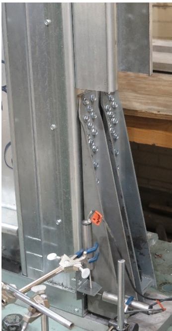
Figure B-12 Centre-sheathed configuration: bottom holdowns (a. & b.) and c. corner of W18-R
