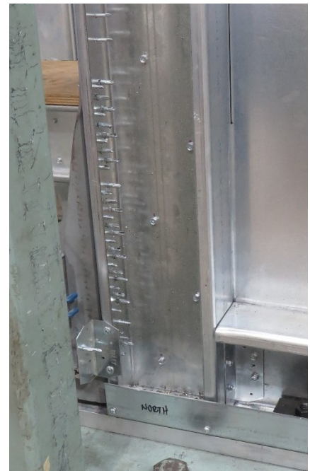
Figure B-12 Centre-sheathed configuration: bottom holdowns (a. & b.) and c. corner of W18-R
