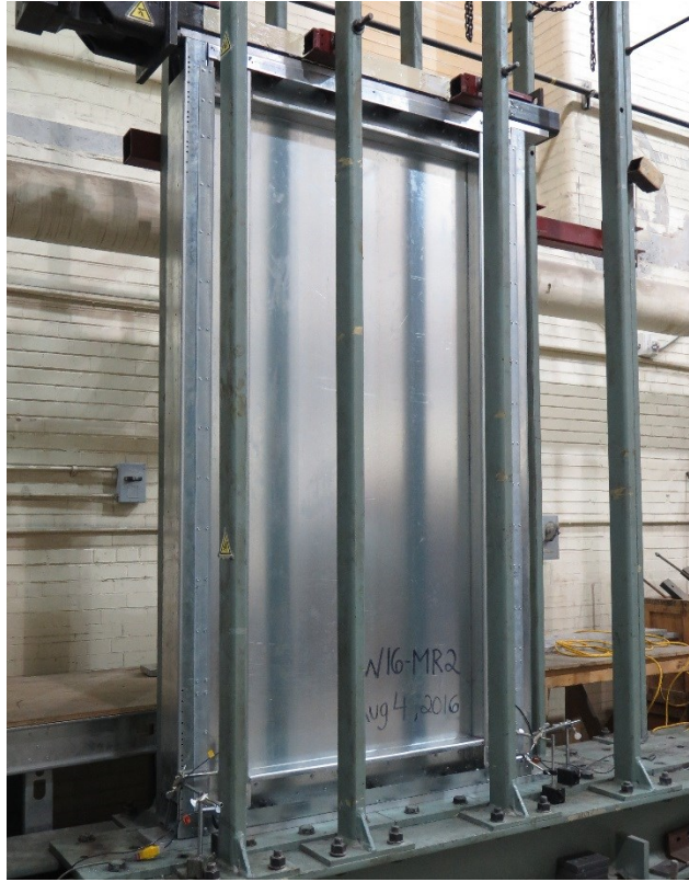
Figure B-13 Centre-sheathed configuration: W16-R2
