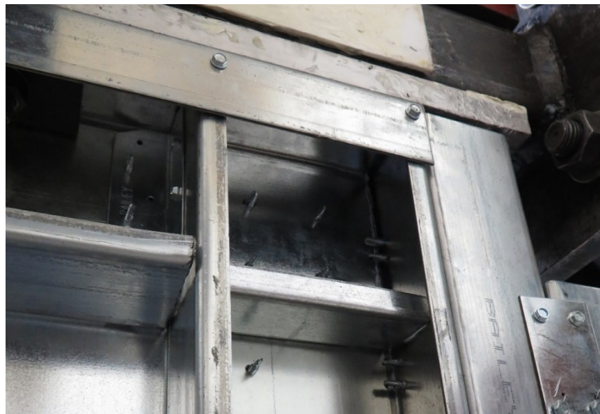
Figure 2.24 Final centre-sheathed configuration: stiffeners added in the corners
