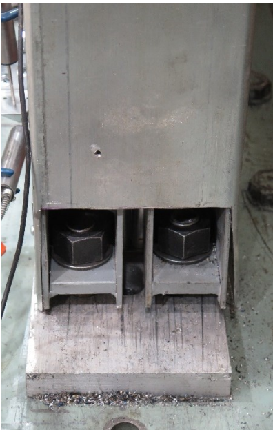
Figure B-14 Centre-sheathed configuration: a. bottom holdowns and b. reinforced corner of W16-R2
