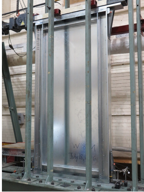
Figure B-9 Centre-sheathed configuration: W18 (unreinforced)
