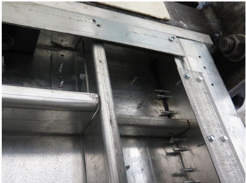
Figure B-14 Centre-sheathed configuration: a. bottom holdowns and b. reinforced corner of W16-R2
