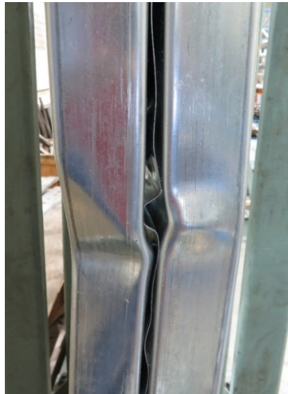
Figure 3.14 Built-up chord studs split due to out-of-plane forces caused by shear buckling of the sheathing
