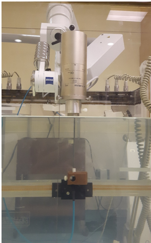
Figure 3-7 – Experimental setup for measurements with the PTW TN60019 microDiamond detector in a Wellhöfer water phantom. The ionization chamber is placed in a plastic holder attached to the Wellhöfer automated 3D scanning system (WP700, version V 3.51.00 , Wellhöfer, Germany).
