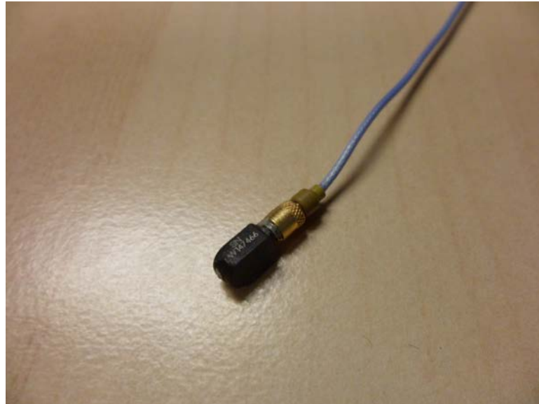
Fig. 3.10 Accelerometer Model 352C23/NC
