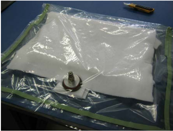
Fig. 4.11 Stage 1 of making a composite plate (layers cut and put in mould)
