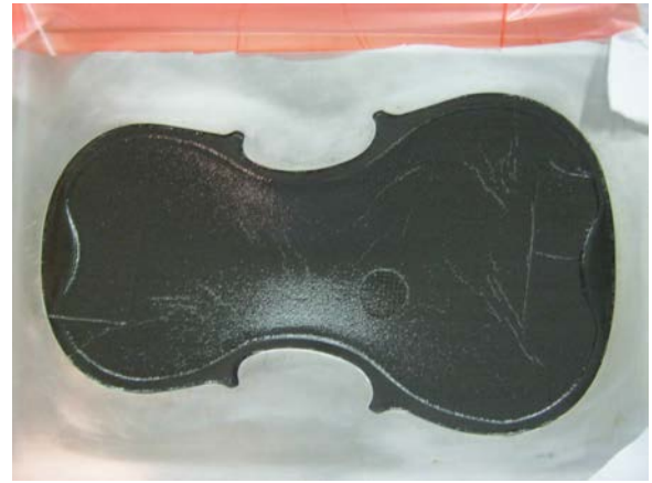
Fig. 4.14 Stage 4 of making a composite plate (after curing)
