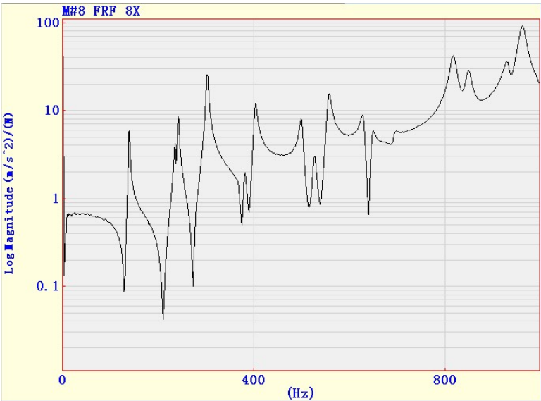
Fig. 5.5 FRF of the spruce plate by the Modal Analysis
