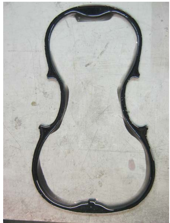
Fig. 4.16 Stage 2 of making the urethane ring
