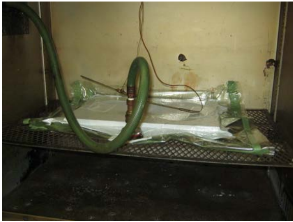
Fig. 4.13 Stage 3 of making a composite plate (vacuum attached)
