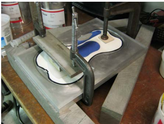
Fig. 4.15 Stage 1 of making the urethane ring
