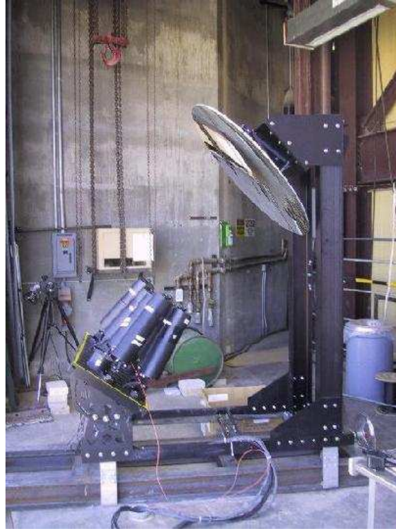
Figure 4.10: Photo of the Southeast PMT camera with its secondary mirror, located on the 220-level of the Solar tower.
