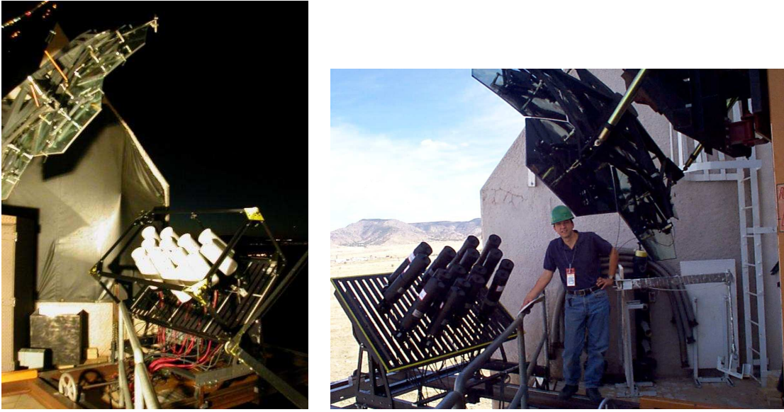
Figure 4.9: Photos of the West ( left ) and East ( right ) PMT cameras with their secondary mirrors, located on the 260-level. The slotted camera plates with adjustable PMT mounts and the faceted secondary mirrors can be seen. (The photo on the right shows the camera in the state before the year 2000, without the box-like metal frame required by the weather protection tarps.) A STACEE collaborator is shown for scale.
