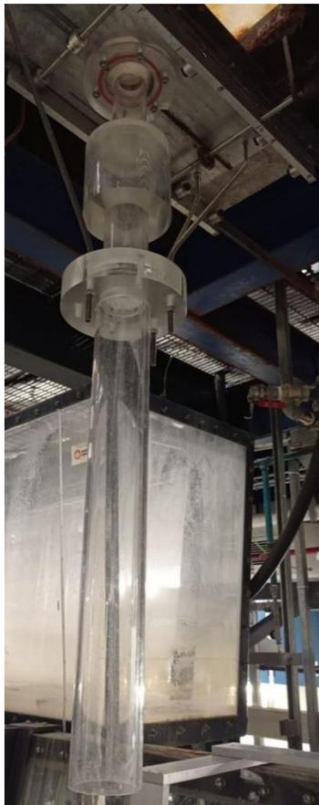
*Figure 59. Ladle Shroud physical model attached to slide gate at the MMPC laboratory.*
