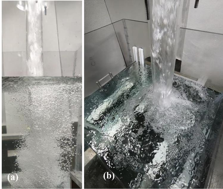
*Figure 79. Air bubbles generated in the liquid in the Tundish-tank surface in (a) front view and (b) isometric view.*
