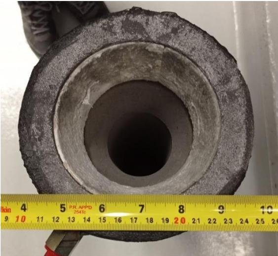
Figure 53. Gasket between the Ladle Shroud and lower nozzle
