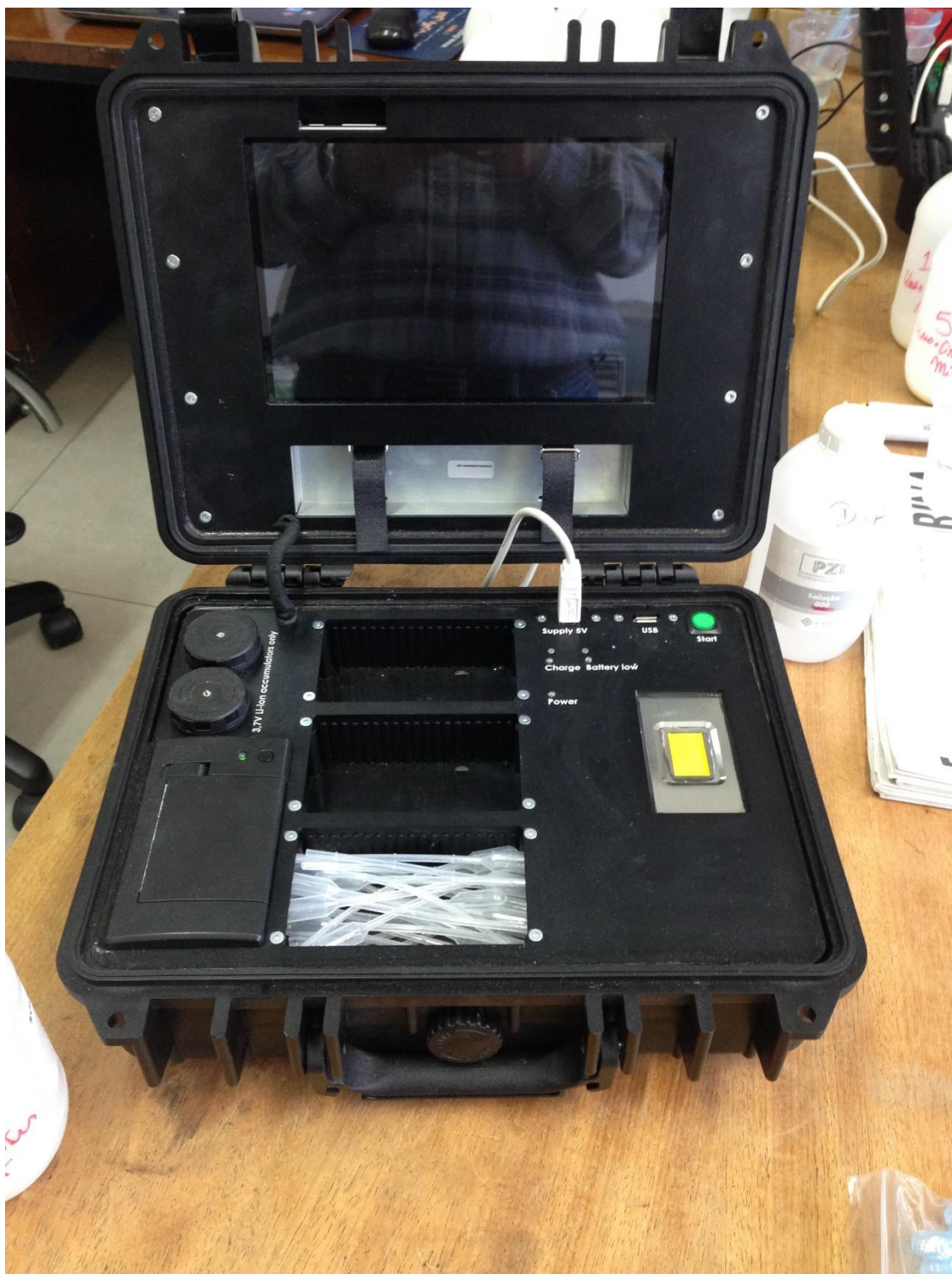
Figure 5-11 Lab-in-Box milk adulteration detector built using LVF ATR-IR spectrometer
