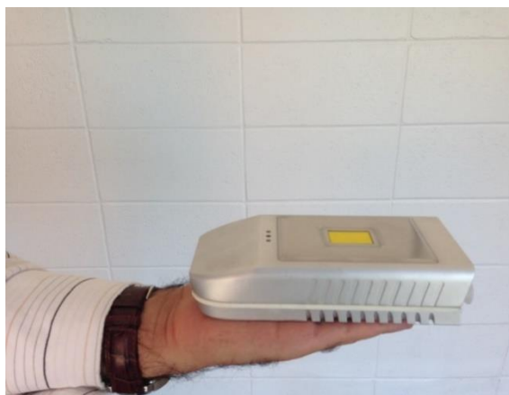
Figure 4-3 IRSphinx (Comline Elektronik Elektrotechnik GmbH, Germany) ATR-IR spectrometer. It does not rely on interferometry to generate different wavelengths. Instead it relies on linear variable filter and pyroelectric line sensor to detect the different IR wavelengths.
