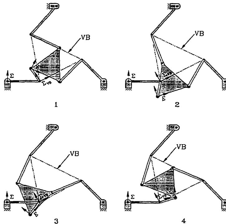
FIGURE A.4. The four real solutions for the RRR example.
