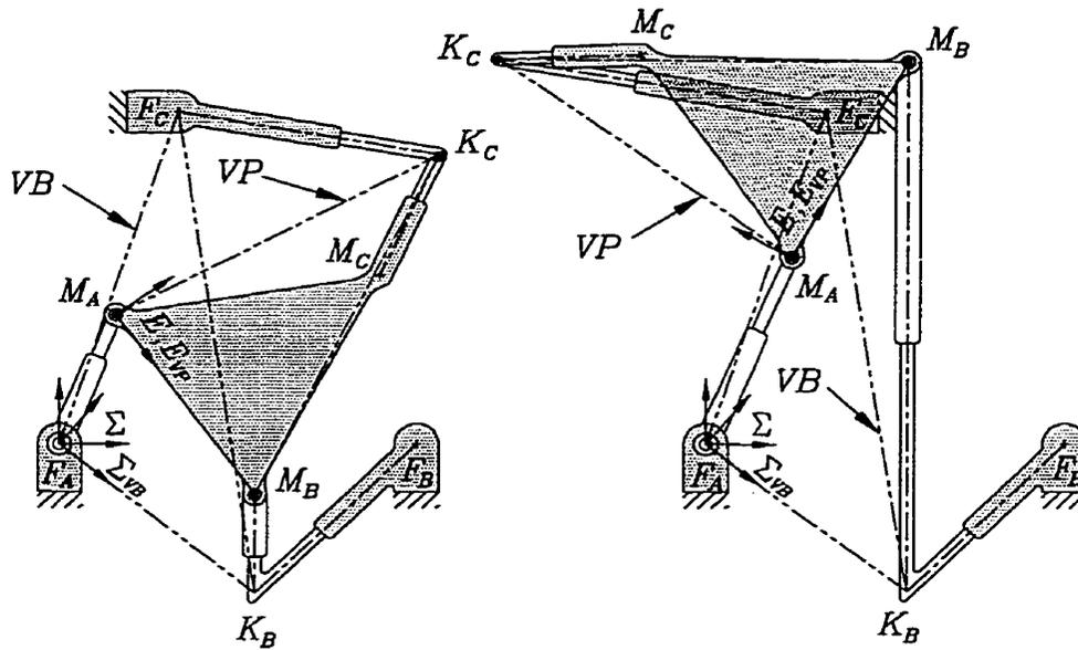
FIGURE A.12. The two real solutions for the mixed PR-type leg example.
