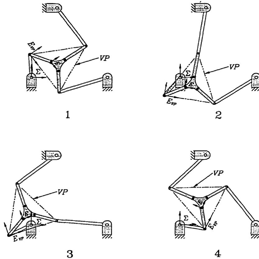
FIGURE A.5. The four real solutions for the RRR example.
