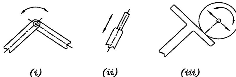
FIGURE 2.1. The three pairs used: (i) *R*-pair; (ii) *P*-pair; (iii) *G*-pair.
