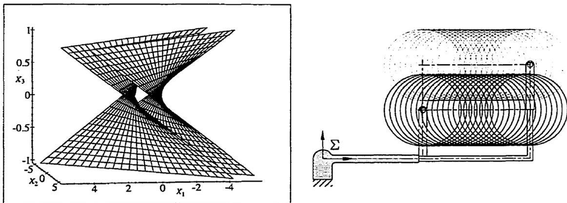
FIGURE 7.5. The kinematic image of the reachable workspace for a *PPR* platform and the corresponding pre-image.
