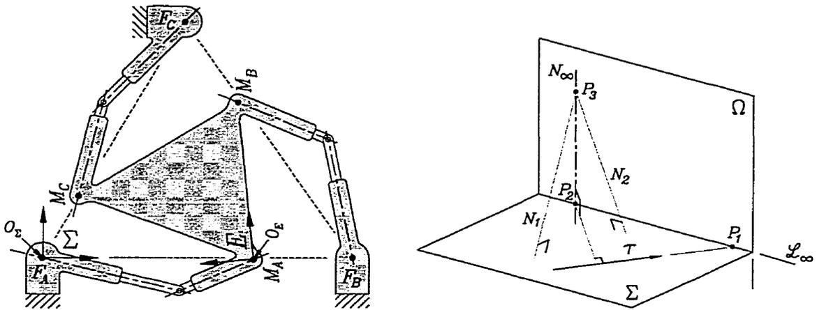
FIGURE 2.6. Reference frames and points where platform joints are  $P$ -pairs; axis associated with a particular  $P$ -pair.
