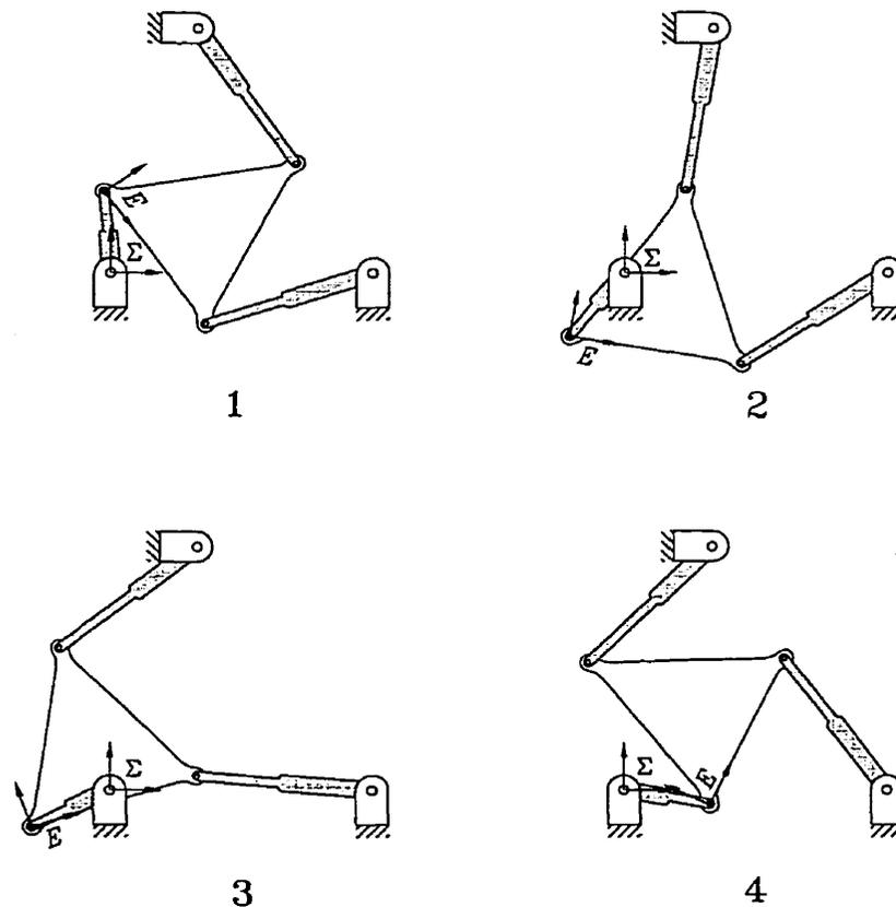
FIGURE A.2. The four real solutions for the Husty *RPR* example.
