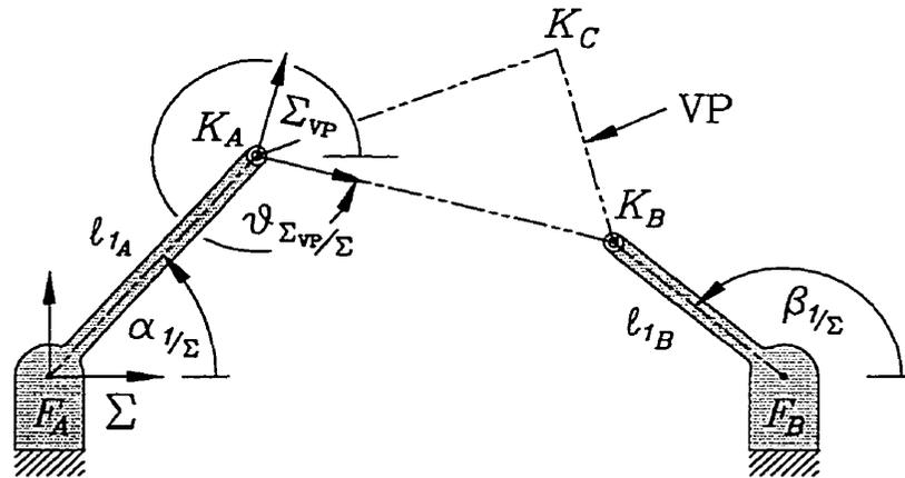
FIGURE 5.10. Determining the VP pose for *RP*-type platforms.
