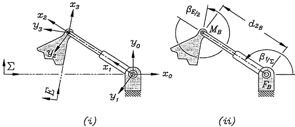
FIGURE 2.12. (i) D-H reference frames in an RPR platform: leg B; (ii) joint parameters.
