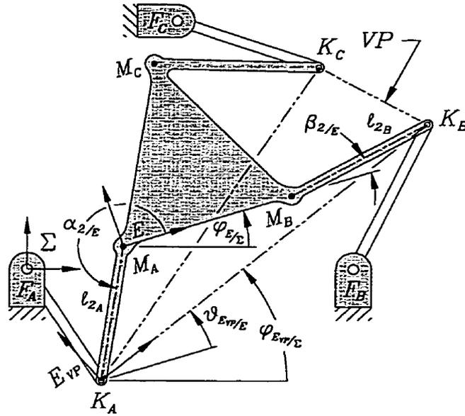
FIGURE 5.9. Determining the VP for PR-type platforms.
