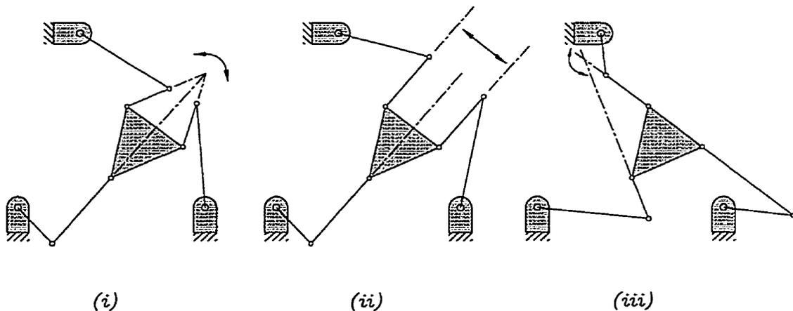
FIGURE 7.8. Three possible  $\underline{RRR}$  platform singular configurations.
