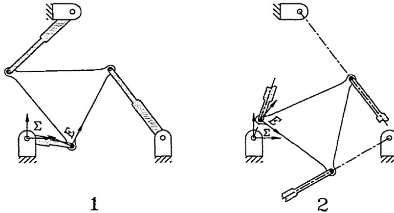
FIGURE A.9. The two real solutions for the  $RPR$  example.
