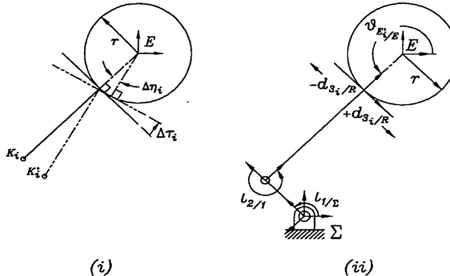
FIGURE 5.12. (i)  $\Delta\tau_i = \Delta\eta_i$ ; (ii) parameters for the  $i^{\text{th}}$  leg.
