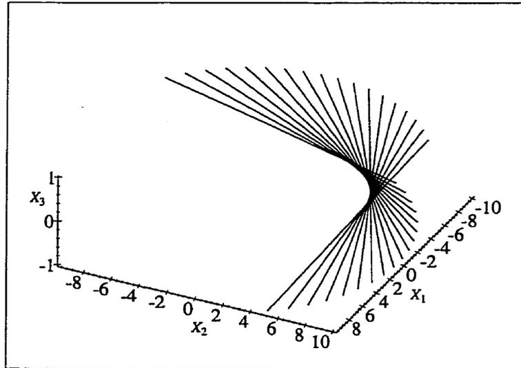
FIGURE 7.7. The set of axes for a set of displacements of one leg of an *RPR* platform.
