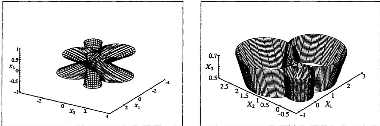
FIGURE A.1. The three constraint hyperboloids for the Husty *RPR* example where  $-1 \leq t \leq 1$  and  $0.5 \leq t \leq 0.7$ , respectively.
