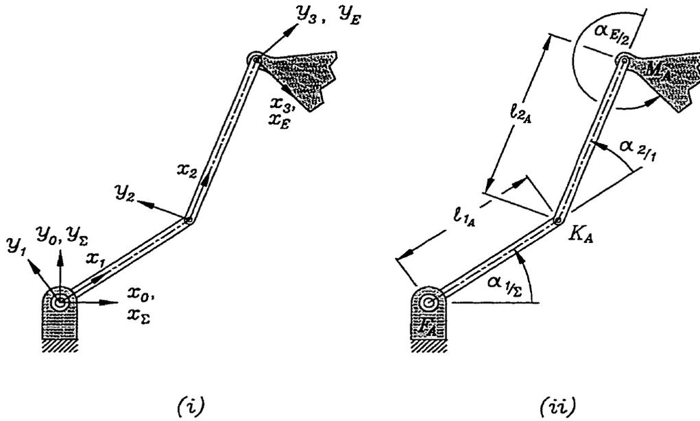
FIGURE 2.11. (i) D-H reference frames in an RRR platform: leg A; (ii) joint parameters.
