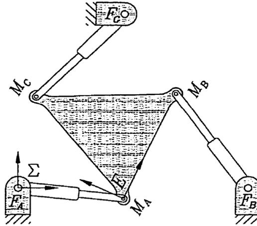
FIGURE 4.6. Convenient reference frames.
