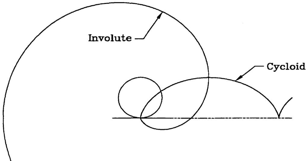
FIGURE 2.8. A cycloid and an involute of a disk.
