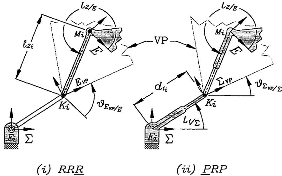
FIGURE 5.8. VP parameters for (i) an RRR and (ii) a PRP platform.
