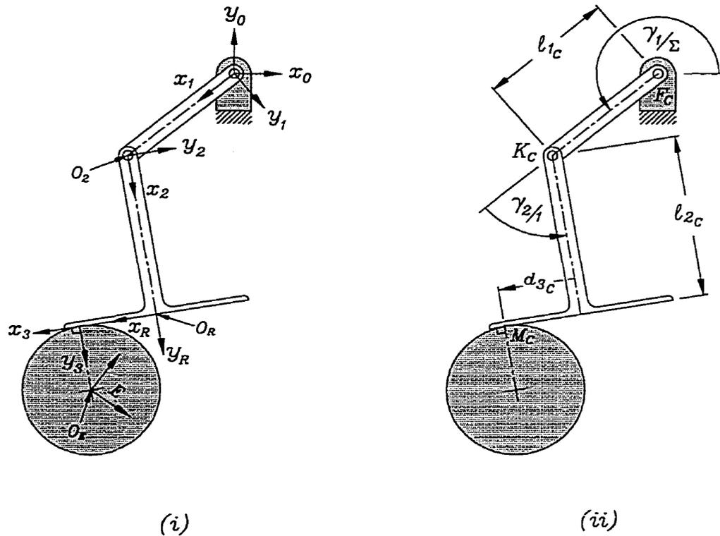
FIGURE 2.14. (i) D-H reference frames in an  $RRG$  platform: leg  $C$ ; (ii) joint parameters.
