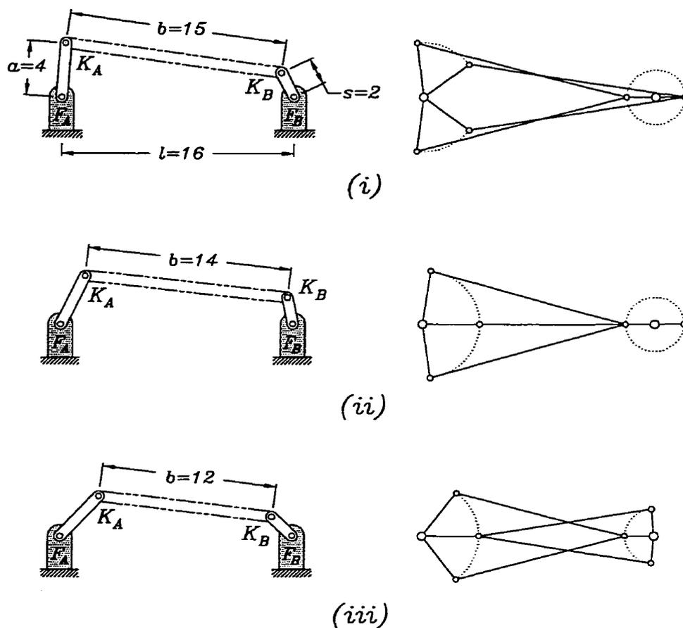
FIGURE 2.9. Application to planar four-bar mechanisms: (i) Grashof; (ii) change-point; (iii) non-Grashof. The excursion arcs and singular positions of the small and large arm crank pins for each of the three cases are shown on the right.
