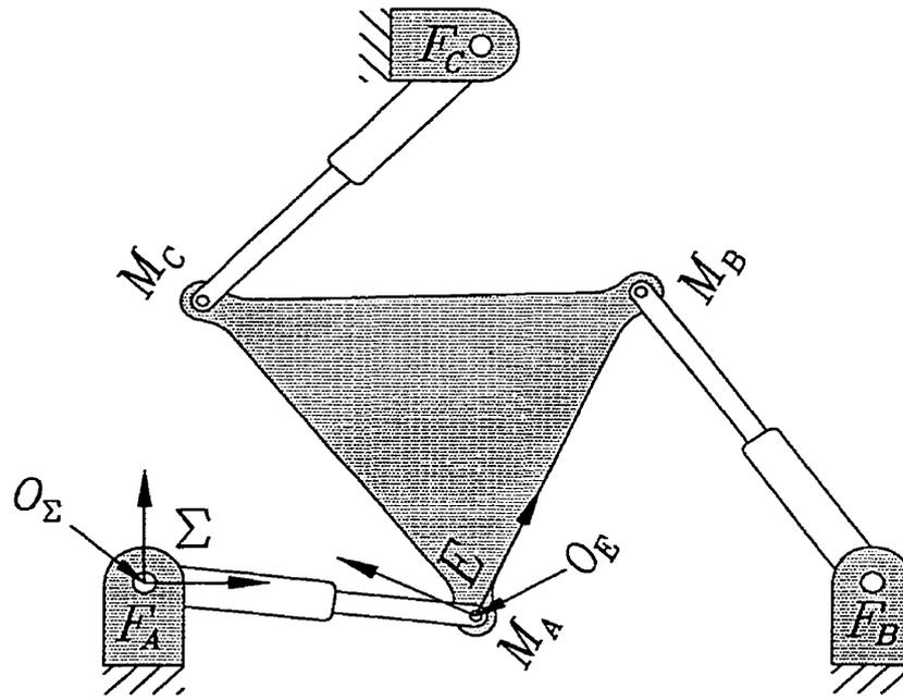
FIGURE 2.5. Reference frames and points if base and platform joints are  $R$ -pairs.
