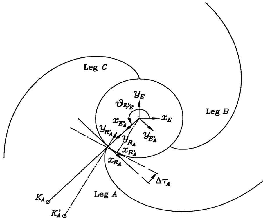
FIGURE 5.14. Reference systems in leg A after a rotation  $\Delta\tau_A$ .
