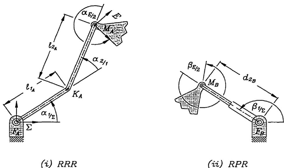
FIGURE 5.1. Parameters for (i) an *RRR* and (ii) an *RPR* platform.
