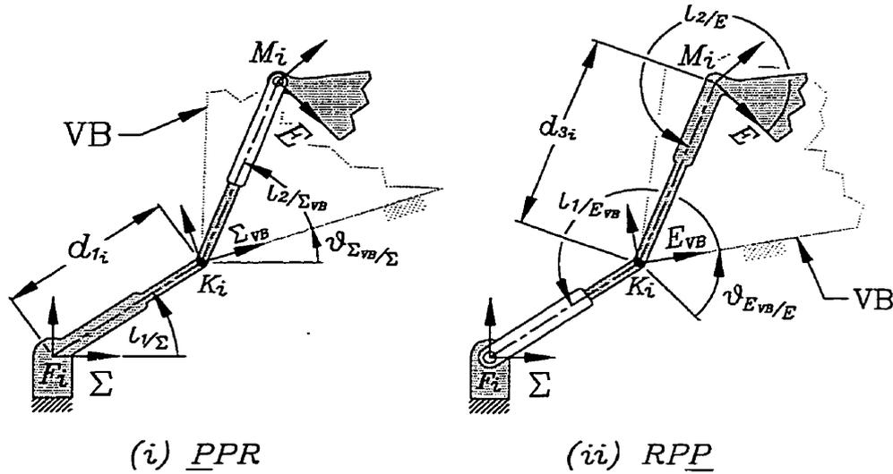
FIGURE 5.3. VB parameters for (i) a PPR and (ii) an RPP platform.
