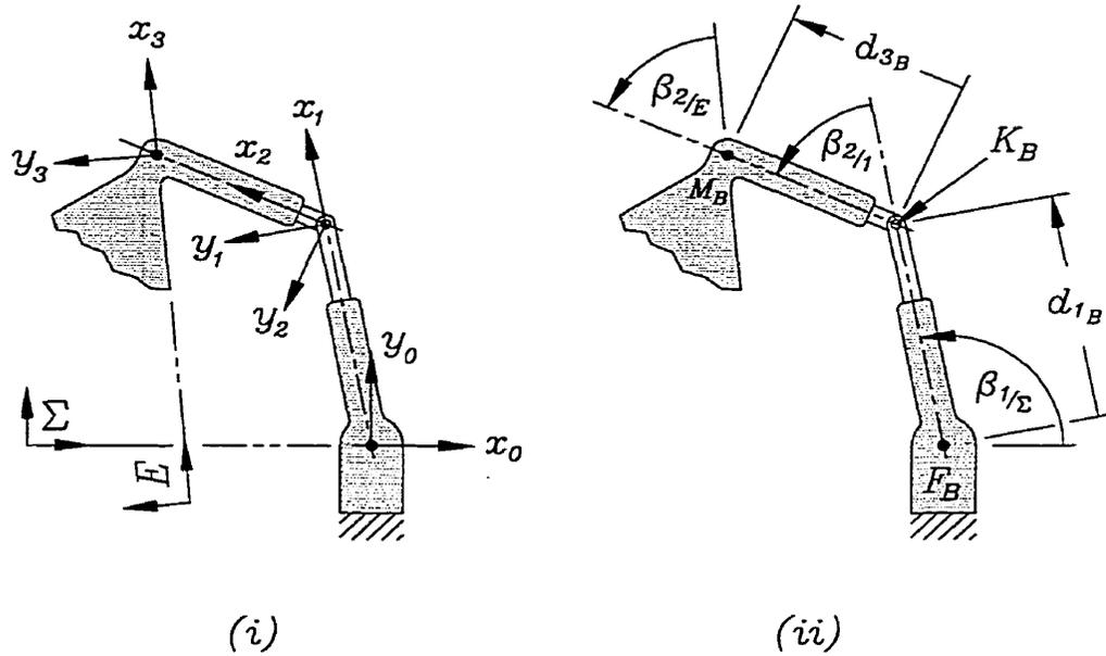
FIGURE 2.13. (i) D-H reference frames in an  $PRP$  platform: leg  $B$ ; (ii) joint parameters.
