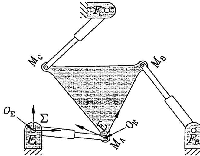
FIGURE 1.6. A typical planar parallel manipulator.
