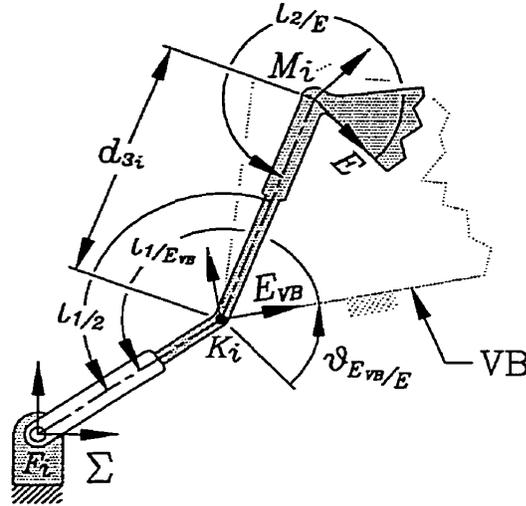
FIGURE 5.7. Determining the VB pose for  $RPP$  platforms.
