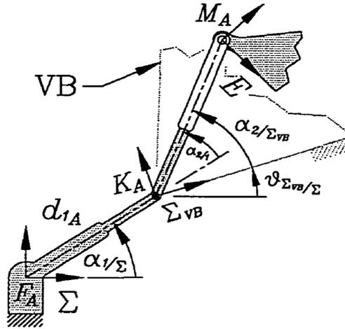
FIGURE 5.5. Determining the VB pose for PPR platforms.
