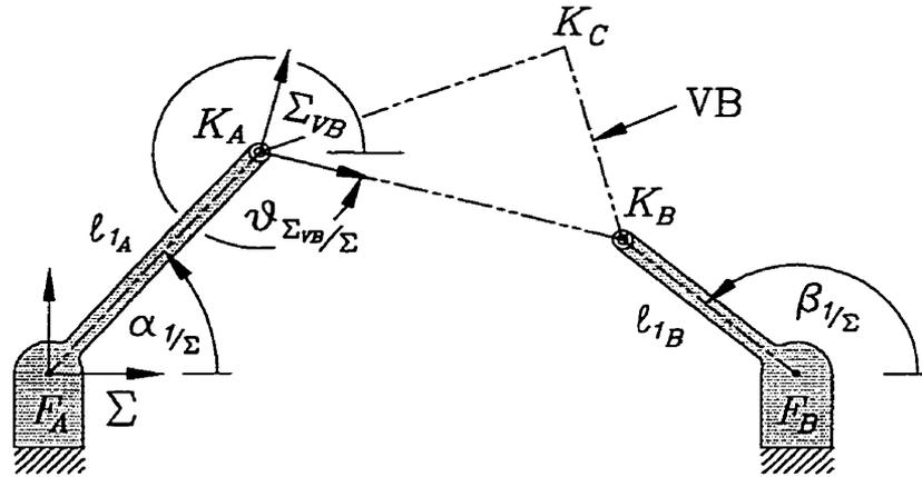
FIGURE 5.4. Determining the VB pose for *RR*- and *PR*-type platforms.
