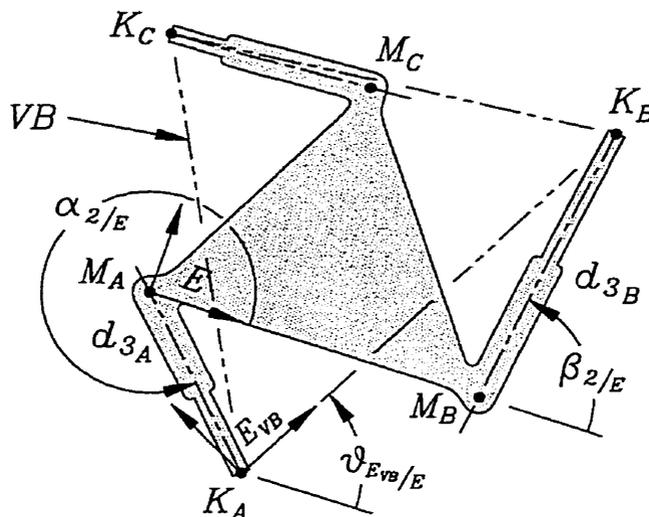
FIGURE 5.6. Determining the VB pose for  $RPP$  platforms.
