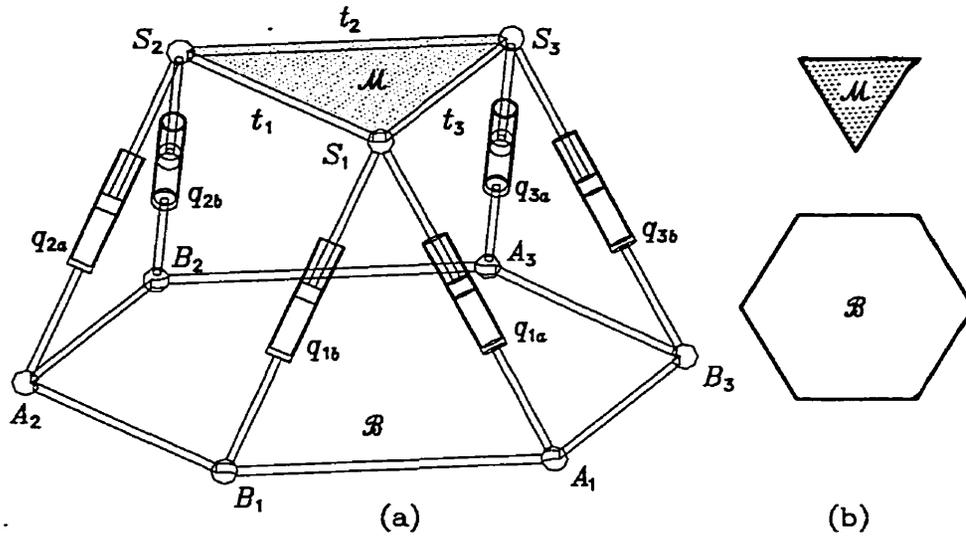
FIGURE 2.2. A UPS-SGP: (a) layout; (b) platform and base geometry (courtesy of Prof. J. Angeles).
