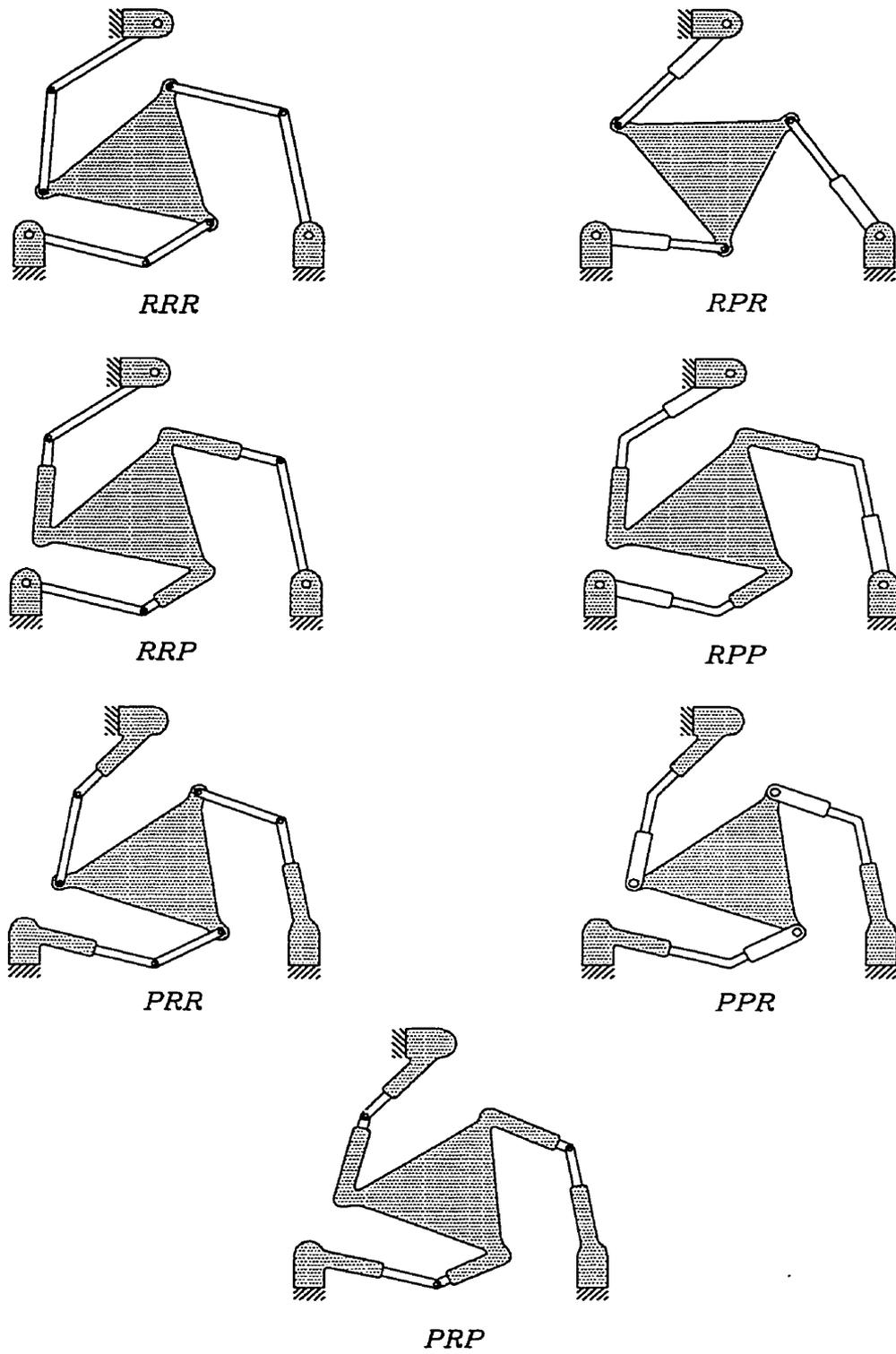
FIGURE 2.4. The seven possible topologies for the PSGP.
