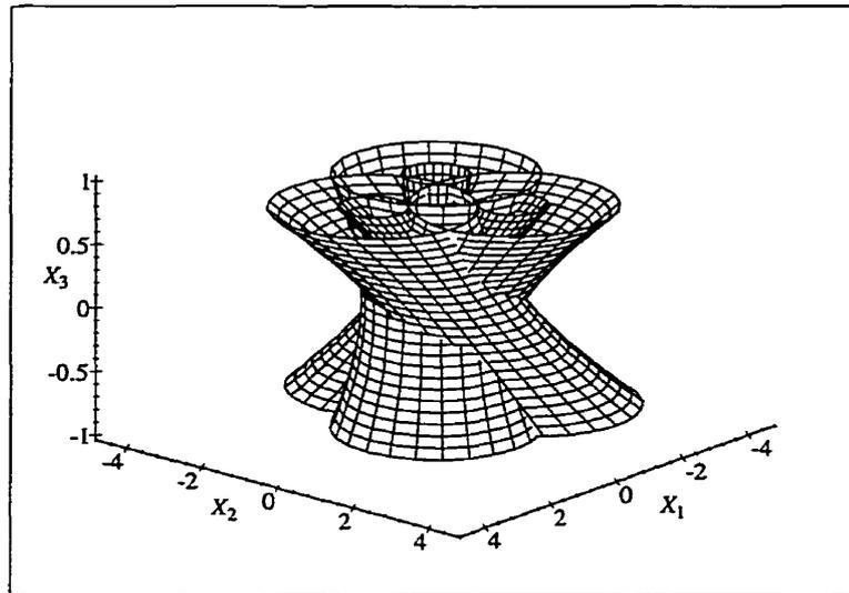
FIGURE 7.2. The kinematic image of the reachable workspace for an  $RPR$  platform.
