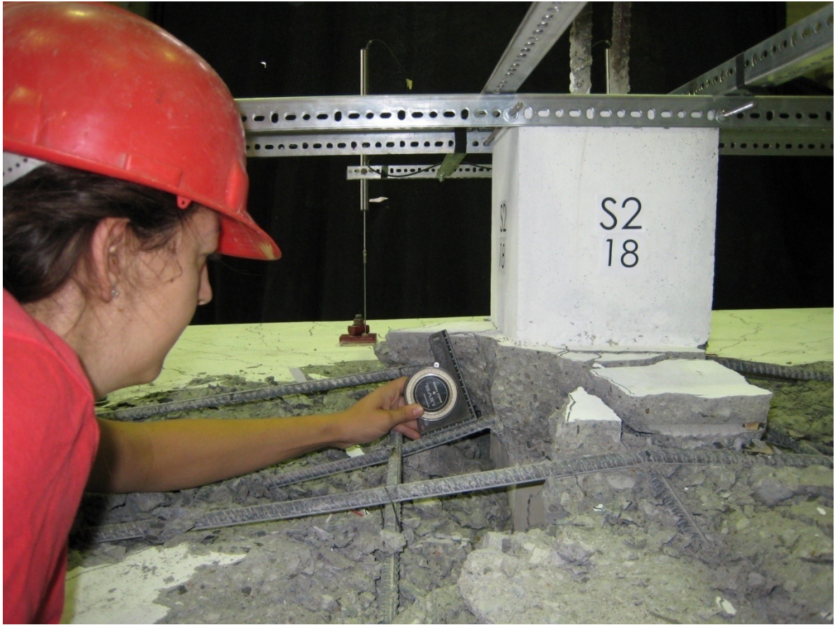
Figure 3.19 Angle of structural integrity reinforcement. Perpendicular bar caused change in angle.
