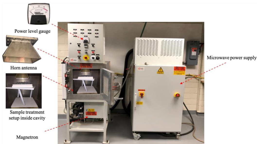
Figure 3-4 Industrial microwave system with variable high power (up to 15 kW) in Geomechanics Laboratory at McGill University
