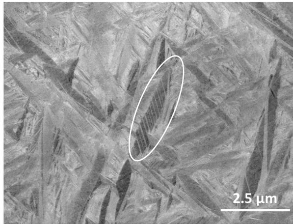
**Fig. 4.4:** ECCI of the powder cross-section of spherical Ti6Al4V powder showing dislocation twins inside the martensitic laths (features inside the white oval).
