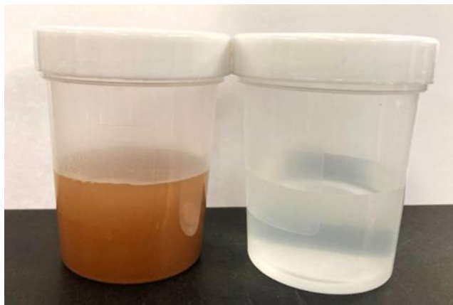
Figure 7.22 - Treated solution with magnetic zeolite particles (left bottle) and after extraction of magnetic zeolite using WHIMS (right bottle).
