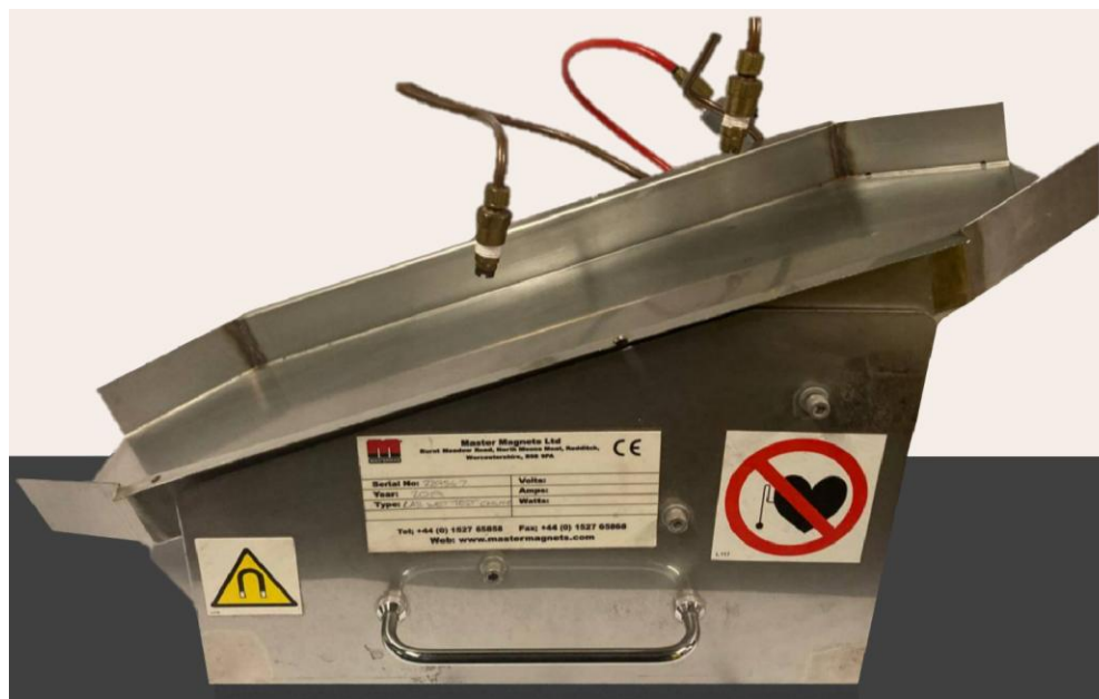
Figure 4.4 - Laboratory wet magnetic test chute.
