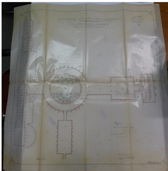
Fig. 2.37 - Plan of the electrical installations running between the Embarcadère and the orangery, signed by Julien Dulait, 1891. The plan specifies the location and type of lamps [Archives du Palais royal, Bruxelles]
