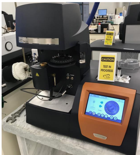
Figure D.16 The thermogravimetric analysis (TGA) Discovery 5500 from TA Instruments.
