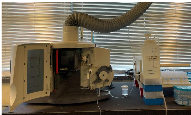
Figure D.11 Thermo Scientific iCAP 6000 Series ICP spectrometer used for ICP-OES testing.
