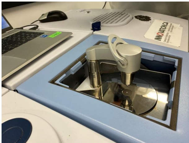
Figure D.14 FTIR infrared spectrometer Vertex 70 from Bruker.
