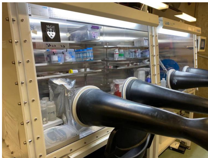
Figure D.3 The Argon-filled glovebox utilized for battery assembling and material preparation.
