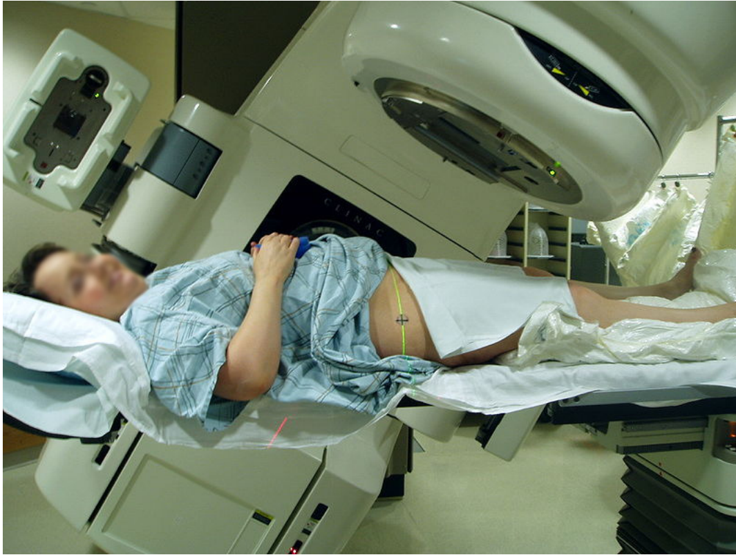
Figure 2-1: Typical linac for external beam radiotherapy. [Author Dina Wakulchik. Reprinted with permission under Creative Commons Attribution 2.0 Generic license]
