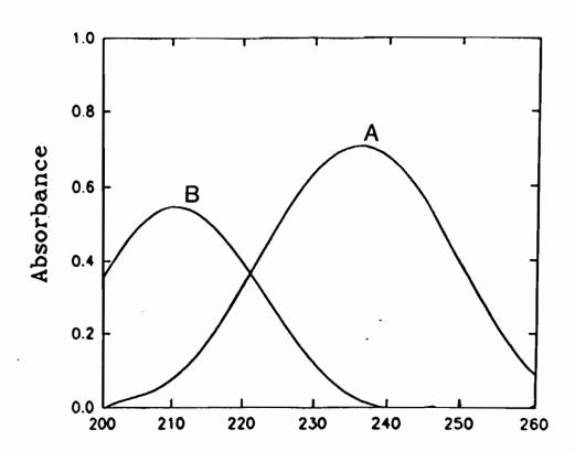
or 210 nm (in 10%  $H_2SO_4$ ) and the amount of PHB over the range indicated (Fig. 8). Although the extinction coefficient decreased from 0.175 ml  $\mu g^{-1} cm^{-1}$  at 235 nm in concentrated  $H_2SO_4$  to 0.143 ml  $\mu g^{-1} cm^{-1}$  at 210 nm in 10%  $H_2SO_4$ , in most cases, when the final concentration of PHB was high enough (> 2  $\mu g/ml$ ) the spectra were recorded in 10%  $H_2SO_4$  as the lower viscosity of these solutions made analyses more convenient.
