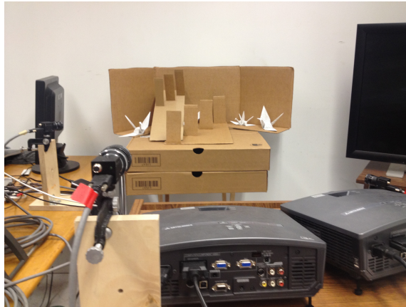
Figure 3-4: Projector-camera experimental setup.
