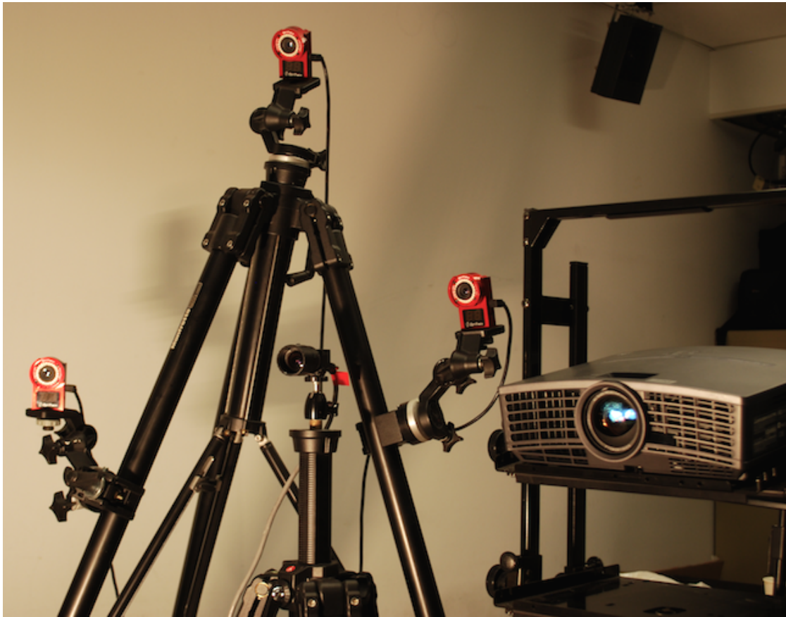
Figure 4–1: Experimental setup. The projector on the right, the three OptiTrack cameras on the left of the image, and the Point Grey camera in front of them are used for the kinetic video projection.
