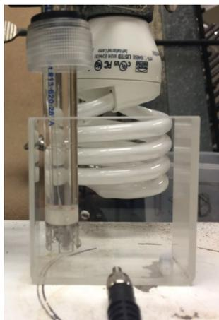
Figure 4.2: Setup for pH cycling experiments.
