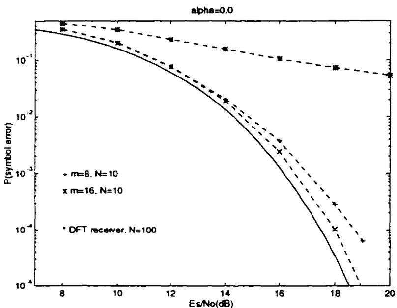
Figure 8.13:  $P(\epsilon) - \frac{E_s}{N_o}$  for 8-PSK,  $\alpha = 0.0$ , with DFT receiver curve.
