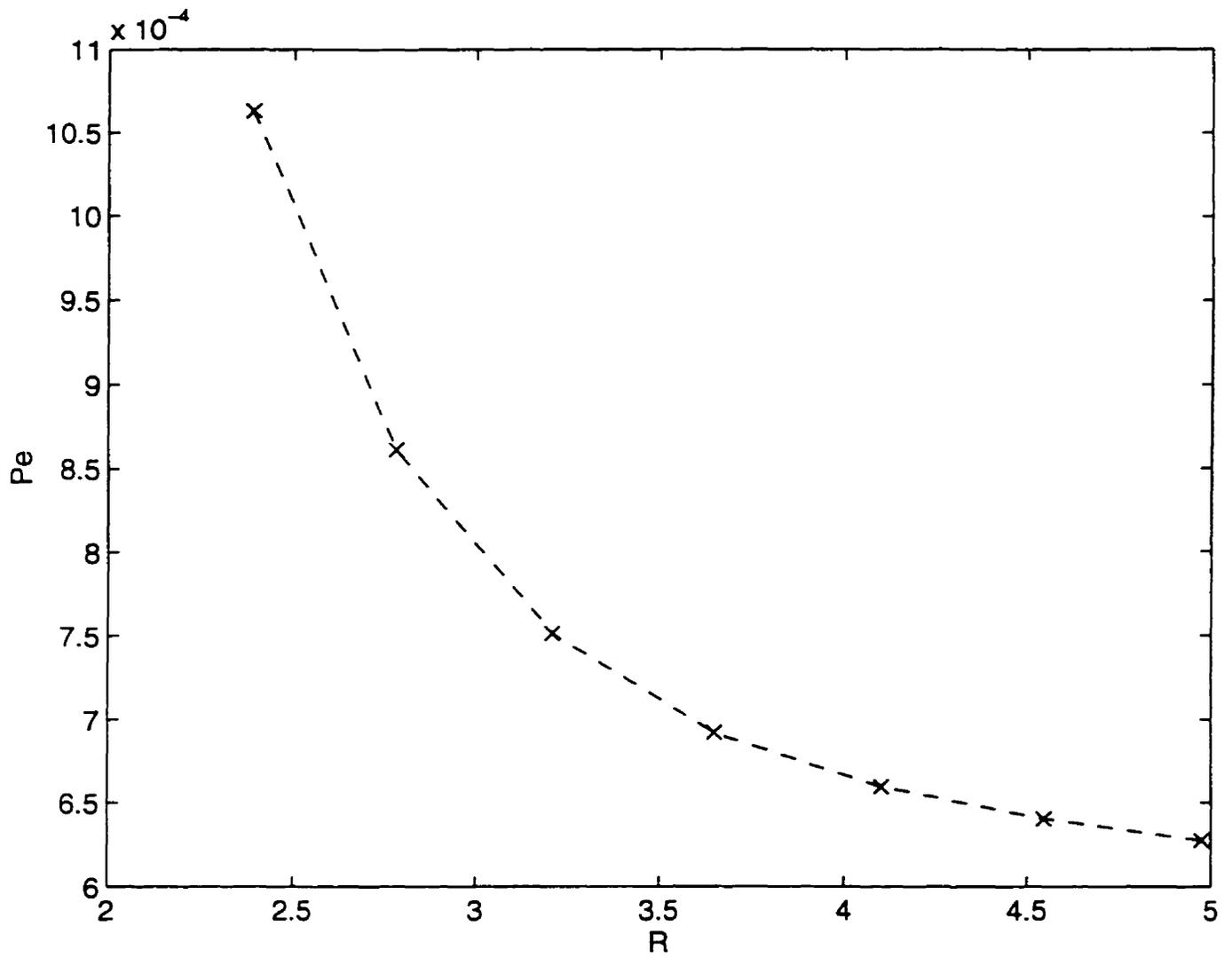
Figure 4.5:  $P(\epsilon)$  vs  $R = \log(m)$  curve for 8-PSK with  $\frac{E_s}{N_0} = 16\text{dB}$
