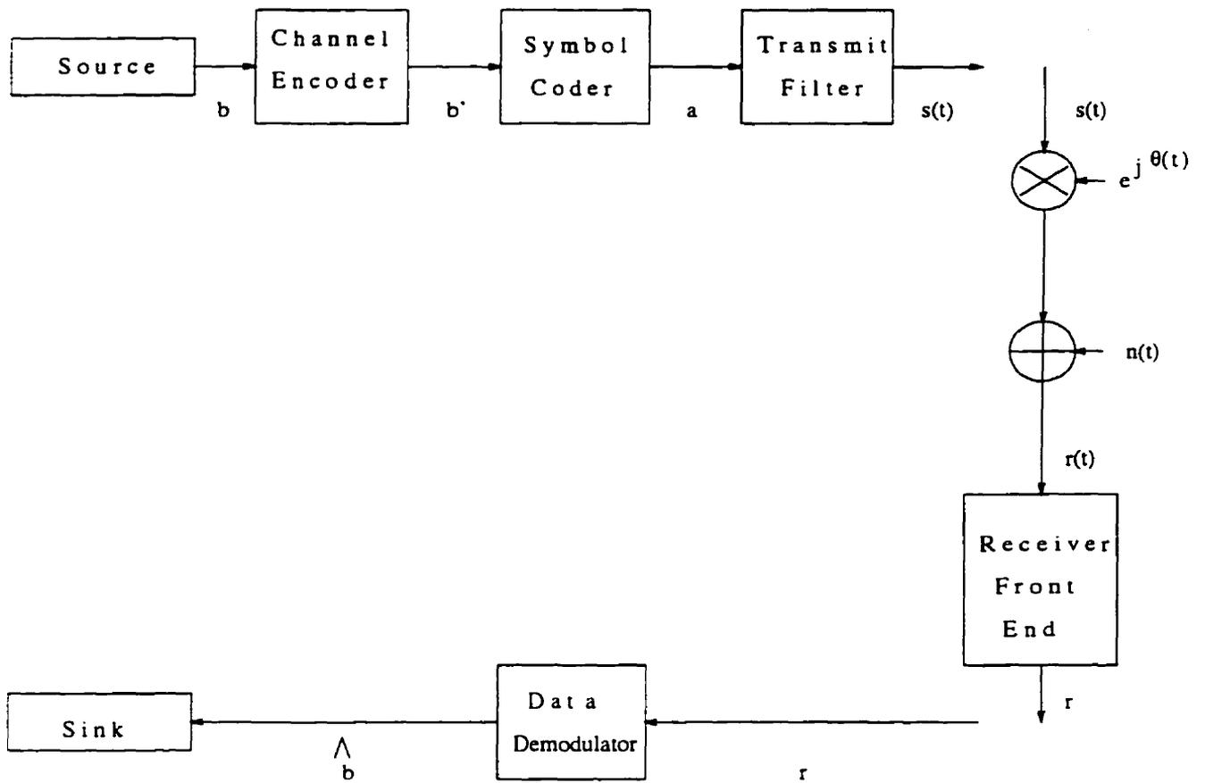
Figure 7.1: The communication system model.
