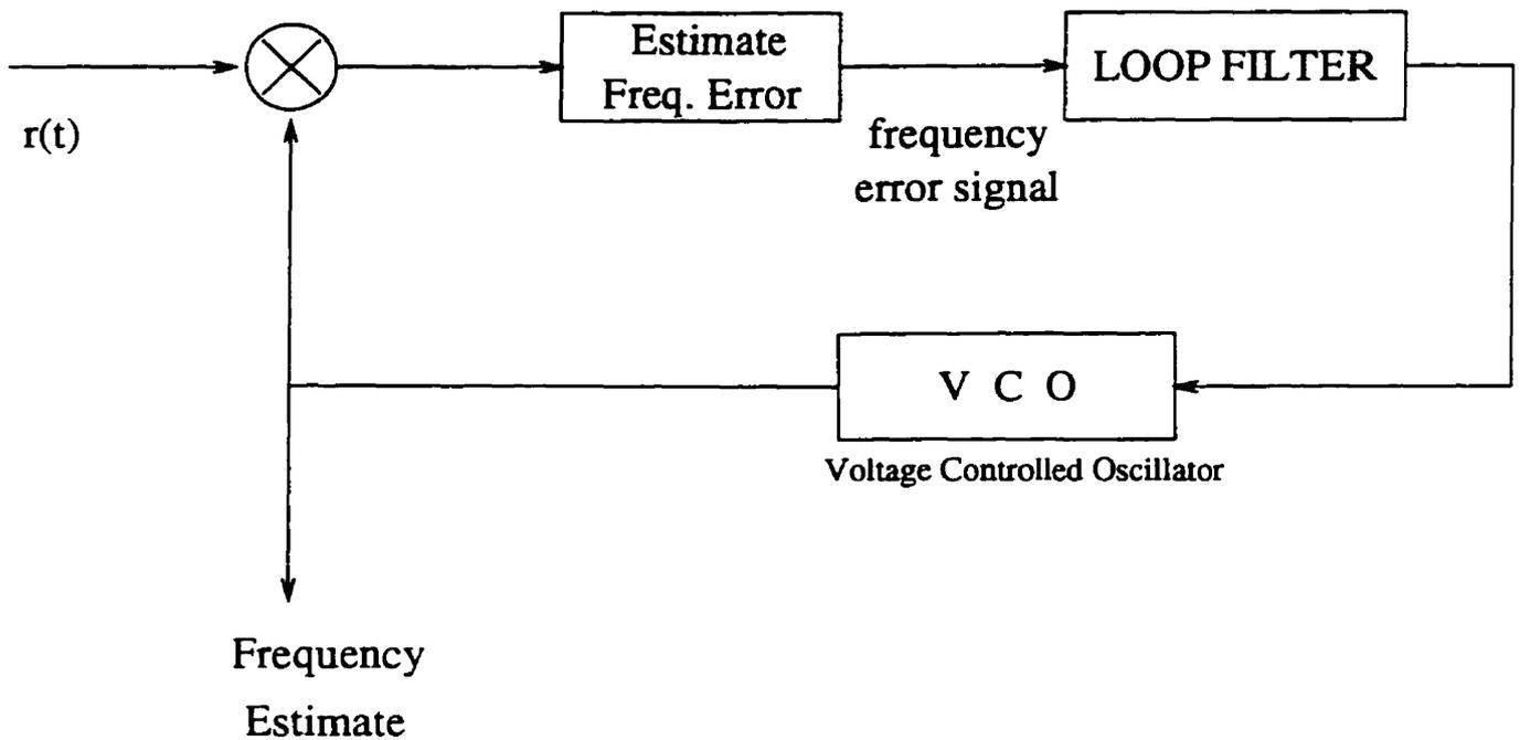
Figure 1.4: Automatic frequency control (AFC) loop.
