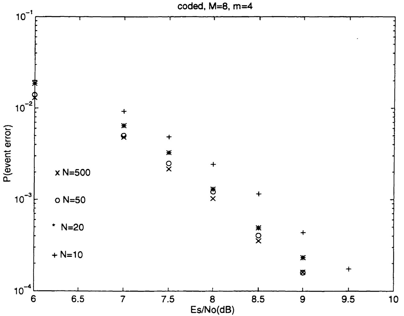
Figure 7.5:  $P(\text{event error}) - \frac{E_s}{N_0}$  curve.
