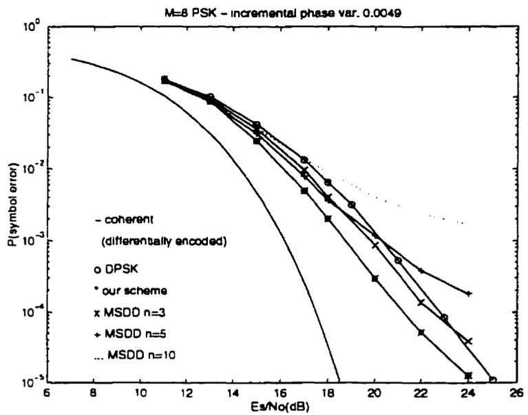
Figure 6.11:  $P(\epsilon) - \frac{E_s}{N_o}$  with  $\sigma = 0.07$ ; also included are MSDD curves.
