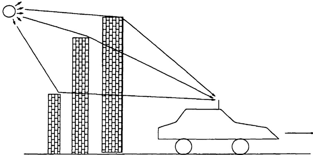
Figure 1.5: The received signal in a mobile communication environment.
