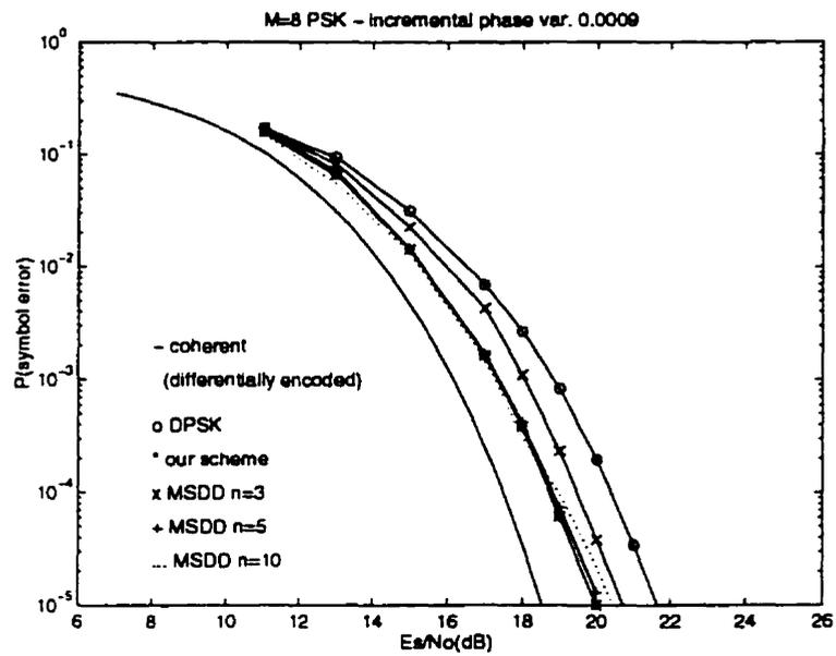
Figure 6.10:  $P(\epsilon) - \frac{E_s}{N_o}$  with  $\sigma = 0.03$ ; also included are MSDD curves.
