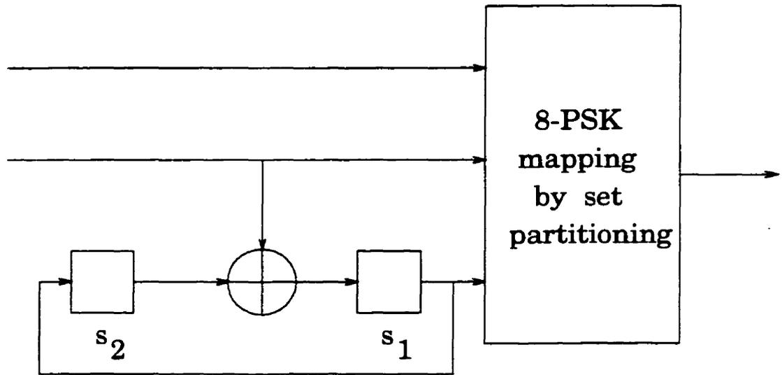
Figure 7.2: Schematic representing the TCM encoding.
