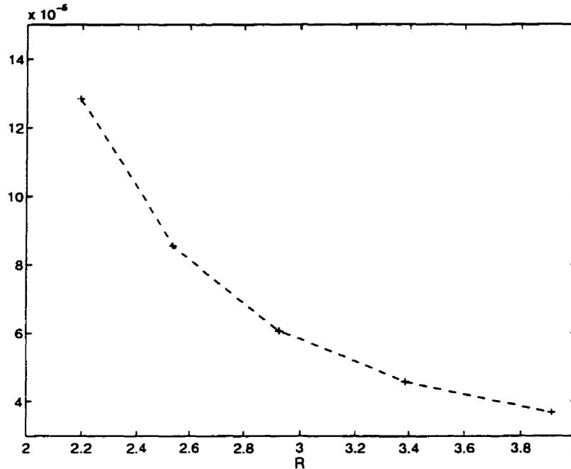
Figure 8.7:  $P(\epsilon)$  vs  $R = \log_2 m$  for QPSK,  $\frac{E_s}{N_o} = 12\text{dB}$ .
