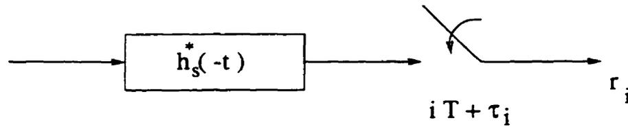
Figure 8.2: A typical receiver front end.
