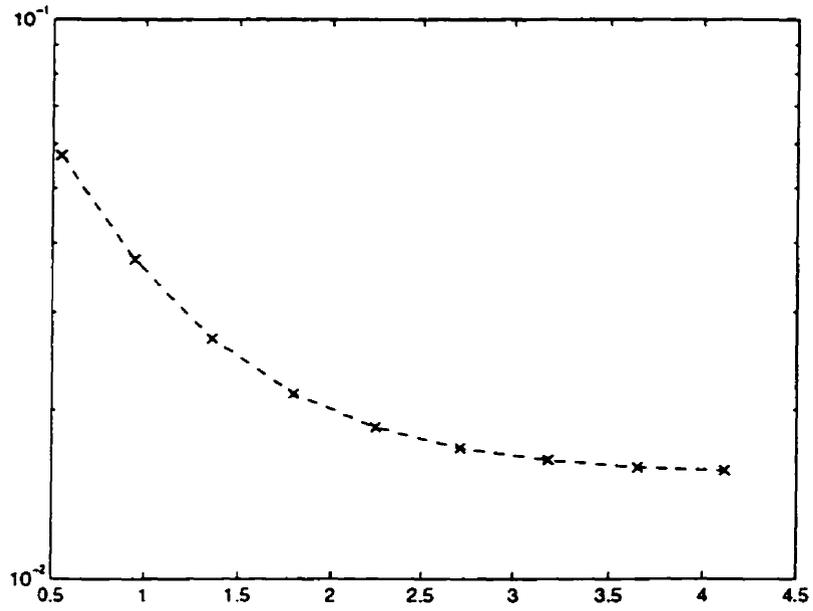
Figure 4.6:  $P(\epsilon)$  vs  $R = \log(m)$  Curve for 8-PSK with  $\frac{E_b}{N_0} = 13\text{dB}$
