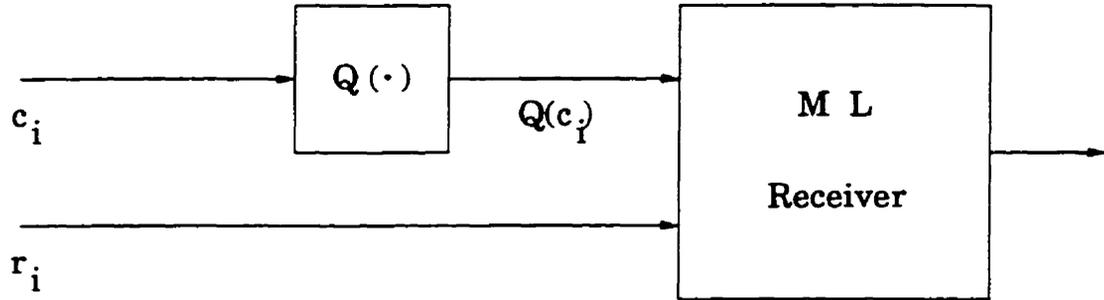
Figure 4.4: Alternative implementation of genie receiver.
