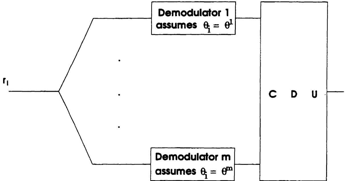
Figure 7.4: Data demodulator implementation.
