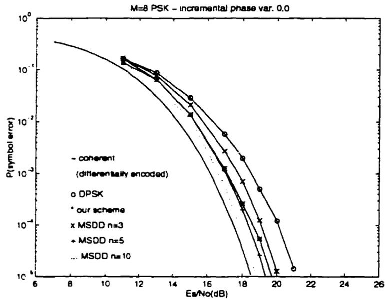
Figure 6.9:  $P(\epsilon) - \frac{E_s}{N_0}$  with  $\sigma = 0.0$ ; also included are MSDD curves.
