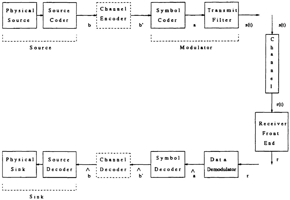
Figure 2.1: The communication system model.
