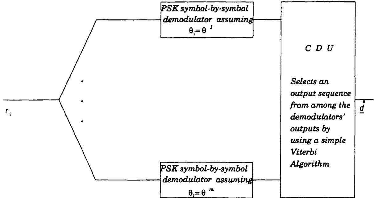
Figure 6.2: The data detector implementation
