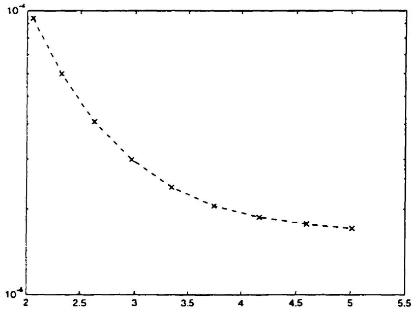
Figure 4.7:  $P(\epsilon)$  vs  $R = \log(m)$  Curve for 8-PSK with  $\frac{E_b}{N_0} = 18\text{dB}$
