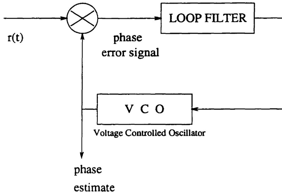
Figure 1.1: A basic phase locked loop (PLL).
