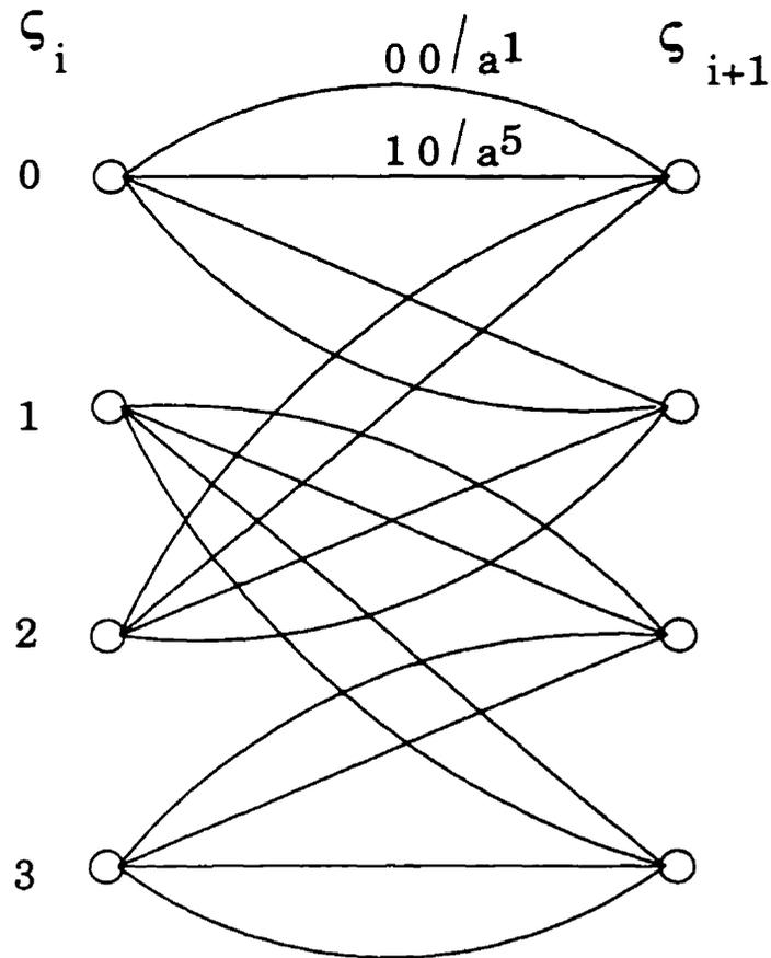
Figure 7.3: Trellis representing the TCM encoding.
