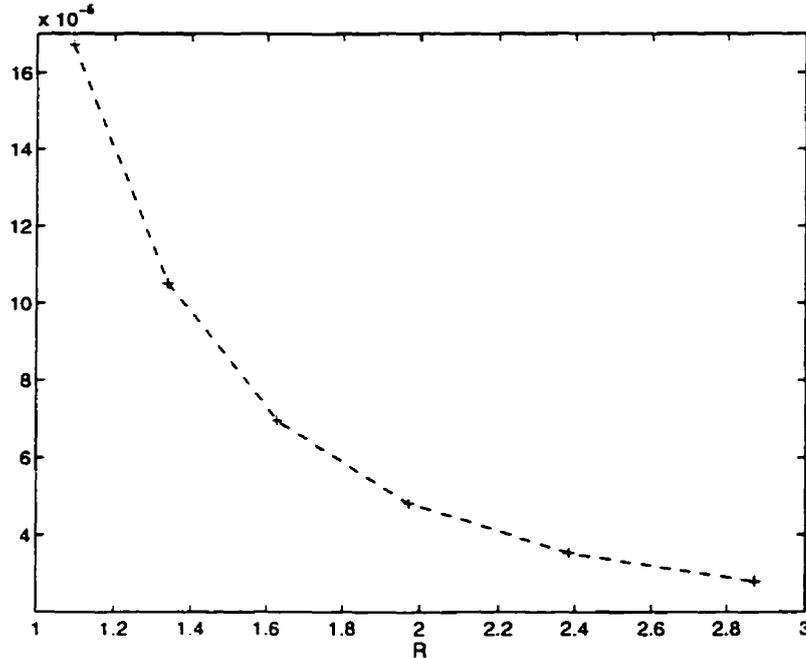
Figure 8.6:  $P(\epsilon)$  vs  $R = \log_2 m$  for BPSK,  $\frac{E_s}{N_0} = 9\text{dB}$ .
