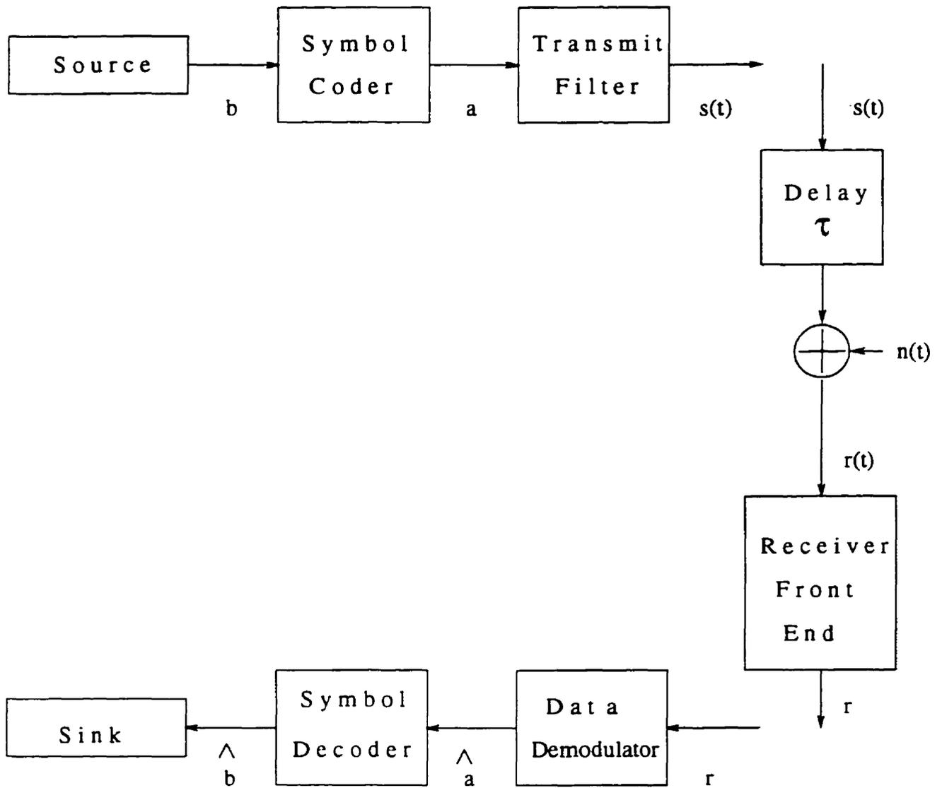
Figure 8.1: The communication system model.
