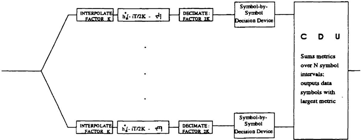
Figure 8.5: The demodulator implementation.
