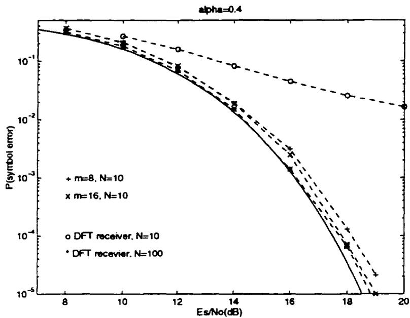
Figure 8.12:  $P(\epsilon) - \frac{E_s}{N_o}$  for 8-PSK,  $\alpha = 0.4$ , with DFT receiver curve.
