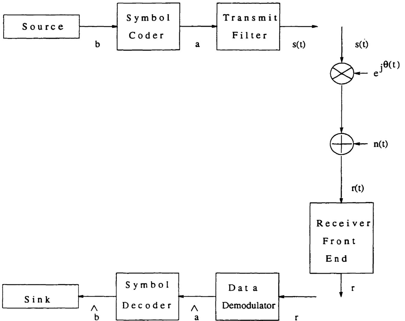
Figure 5.1: The communication system model
