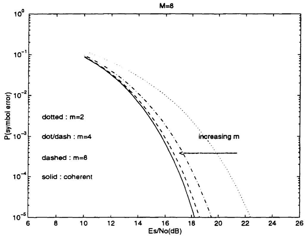
Figure 4.8:  $P(\epsilon) - \frac{E_s}{N_0}$  as a function of  $m$  for 8-PSK
