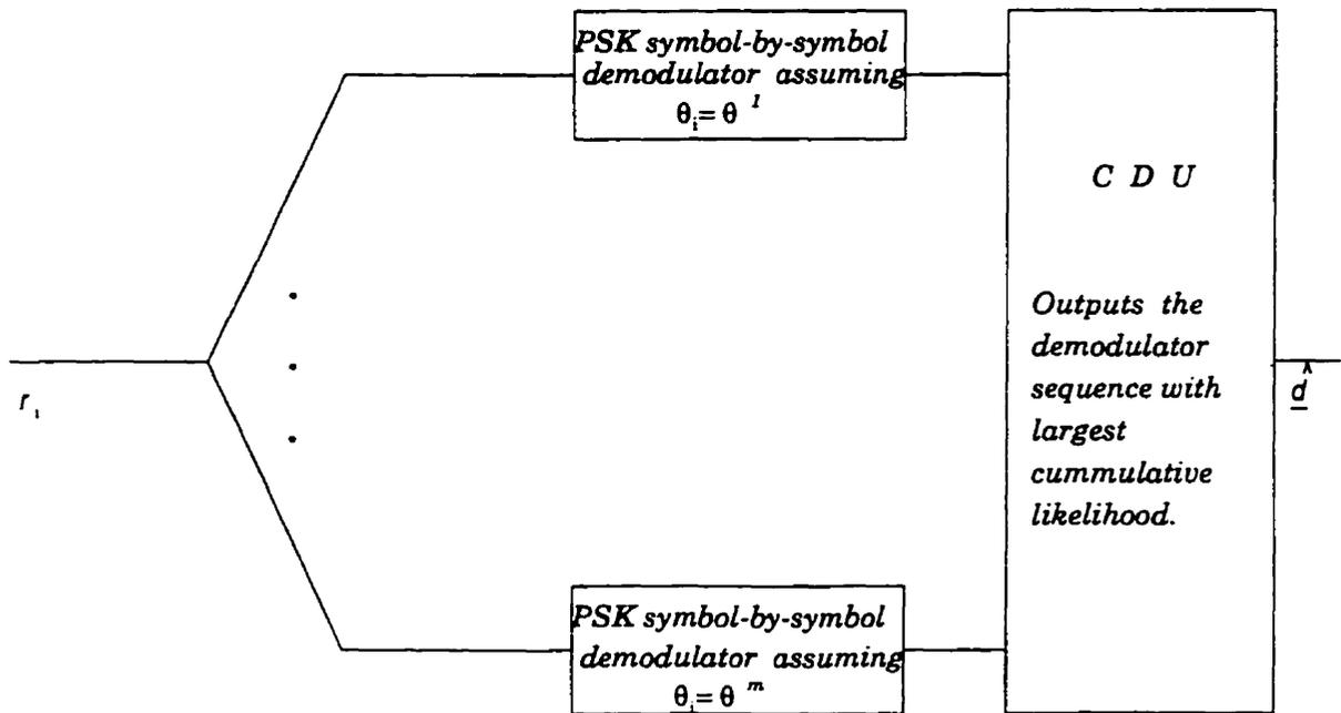
Figure 5.2: The data detector implementation.
