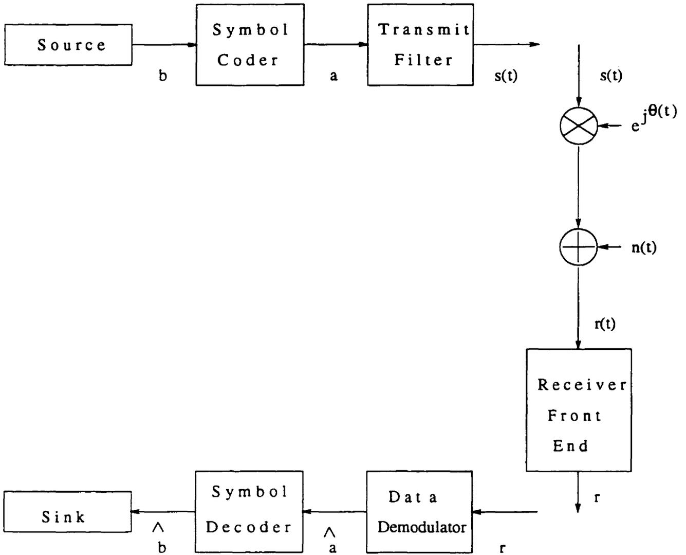
Figure 6.1: The communication system model.
