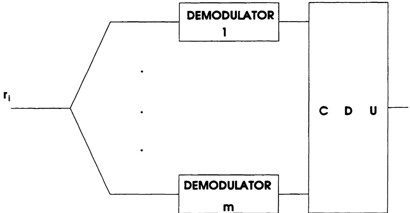
Figure 3.1: The general receiver structure.
