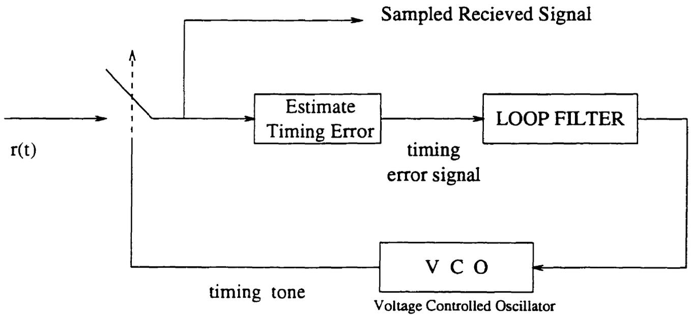
Figure 1.3: Inductive timing recovery.
