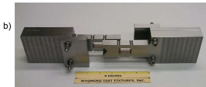
Figure 25: Open Hole Compressive Test Fixture (a) Isometric View [20] (b) Isometric Picture 9
