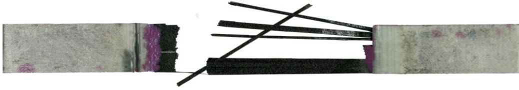
Figure 47: Typical Tensile fracture for a coupons without defect
