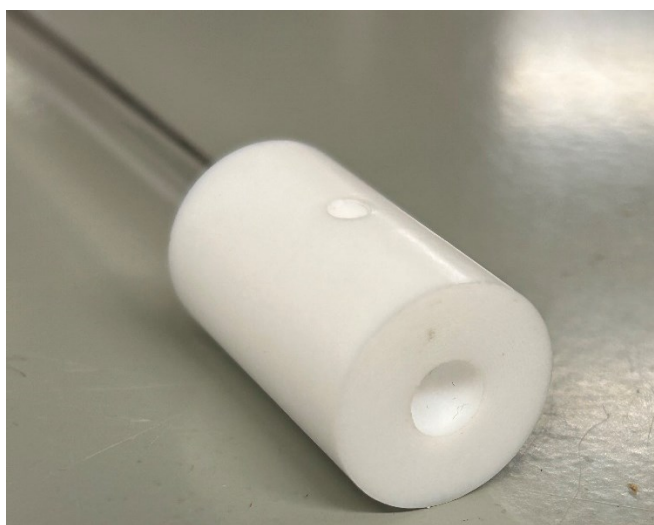
Figure 35: Tube attachment prototype to facilitate in-flight functionalization in air
