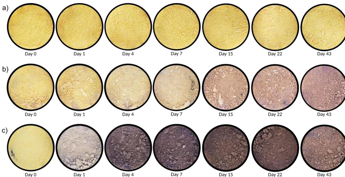
**Figure 2.7** Macroscopic photos showing the changing color of the milled powders over the aging period. Powders were aged at a)  $-18\text{ }^{\circ}\text{C}$ , b)  $21\text{ }^{\circ}\text{C}$ , and c)  $32\text{ }^{\circ}\text{C}$ .
