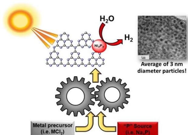
**Figure 1.6** Abstract figure for the mechanochemical synthesis of nickel phosphide nanoparticles and the HER catalyzation application. Reprinted with permission from Ref. 56. Copyright 2020 American Chemical Society.<sup>56</sup>
