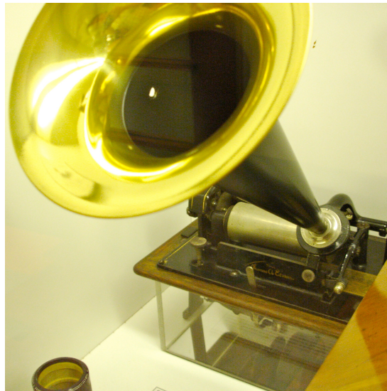
Figure 2.7: Early wax cylinder recording apparatus (image from Nascè 2009, 11)
