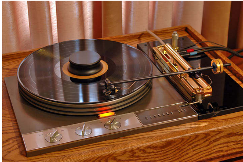
Figure 2.18: A turntable with its linear tracking tonearm (Eugenio, 2010)
