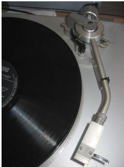
Figure 2.19: A turntable with its pivoted tonearm (Wikipedia, 2011)
