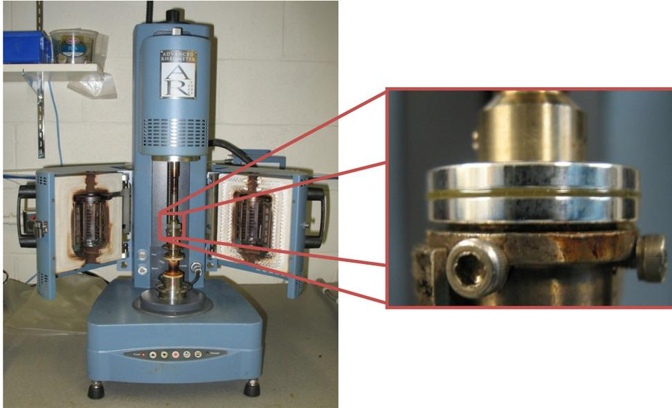
Figure 3.14: Rheometer with close-up of the parallel plate geometry.
