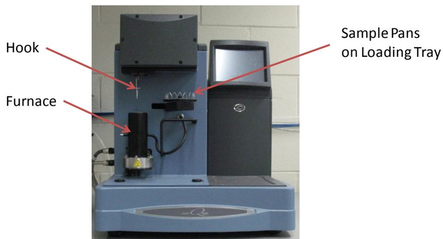
**Figure 3.1 The Thermal Gravimetric Analyzer.**
