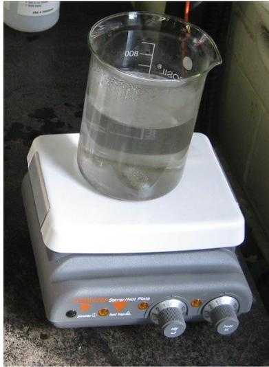
Figure 5.6: Hot water submersion test setup.
