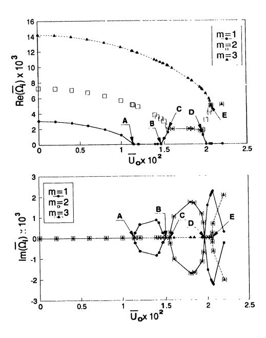
Figure 4.6: Typical Argand diagram involving the real,  $\text{Re}(\bar{\Omega}_t)$ , and imaginary,  $\text{Im}(\bar{\Omega}_t)$ , parts of the dimensionless eigenfrequencies of the so-called 1/10-gap system with viscous annular water flow and a stagnant internal fluid (water), as the dimensionless annular flow velocity  $\bar{U}_o$  is varied, when the outer cylinder is rigid and the inner shell (steel) is pinned-clamped; for  $n=3,\ m=1,\ 2$ .
