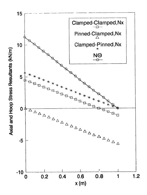
Figure 4.10: Comparison between stresses induced by annular viscous flow in the case of pinned-clamped or clamped-pinned system and those in the case of clamped clamped system.
