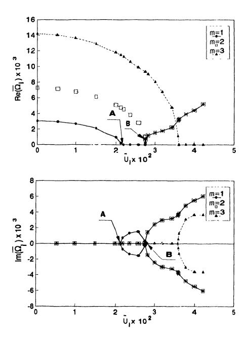
Figure 4.2: The real and imaginary parts of the dimensionless eigenfrequencies,  $\bar{\Omega}_{ij}$ , of the 1/10-gap system (see equation (4.1)) with viscous internal water flow and a stagnant annular fluid (water), as functions of the dimensionless inner flow velocity,  $\bar{U}_{ij}$ , when the outer cylinder is rigid and the inner shell (steel) is pinned-clamped; for n=3, m=1, 2, 3.
