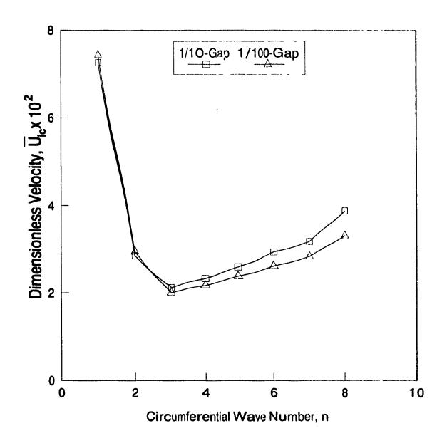
Figure 4.4: The effect of L/c on the overal! (lowest) critical dimensionless flow velocity,  $\bar{U}_{ic}^*$ , for the 1/10-gap system conveying internal water flow and quiescent annular fluid (water); the circumferential wave number n associated with the first loss of stability is shown in the figure. The system is pinned-clamped.
