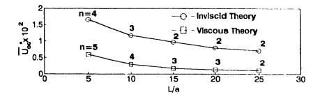
Figure 4.8: The overall critical dimensionless annular flow velocity,  $U_{oc}^*$ , in the 1/10-gap system as a function of the dimensionless wall-thickness of the shell  $h_i/a$ , with the circumferential mode, n, associated with the first loss of stability indicated in the figure. The shell (steel) is pinned-clamped and the inner fluid (water) is stagnant.
