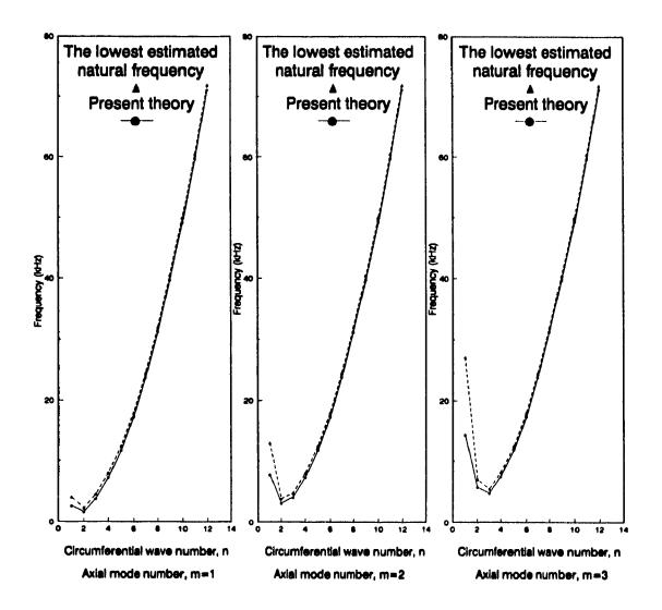
Figure 3.2: Comparison between the lowest natural frequencies of a pinned-clamped shell (steel) conveying internal fluid (water) with dimensionless velocity  $\bar{U}_i$ , as calculated by beam theory with one comparison function (M=1) and by the present theory with three comparison functions (M=3), for circumferential wave number n=1 and axial mode number m=1.
