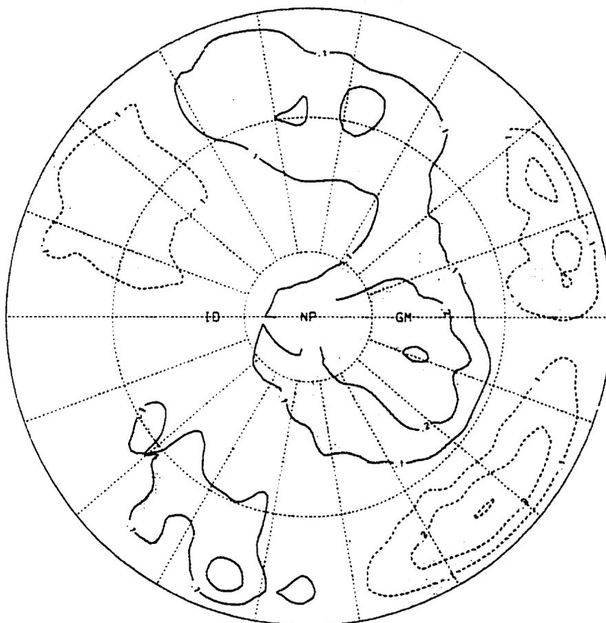
Figure 15: Spatial map of temporal lagged-correlation coefficients between the SVD<sub>1</sub>(SIC) expansion coefficient and the time series of the SLP anomalies at each grid point, with atmosphere leading SVD<sub>1</sub>(SIC) by 1 year. The latitude circles shown are for 45°N, 60°N and 80°N, the dotted line cross the N.P is the dateline. The shaded parts represent regions where correlations are significant at 95% level.
